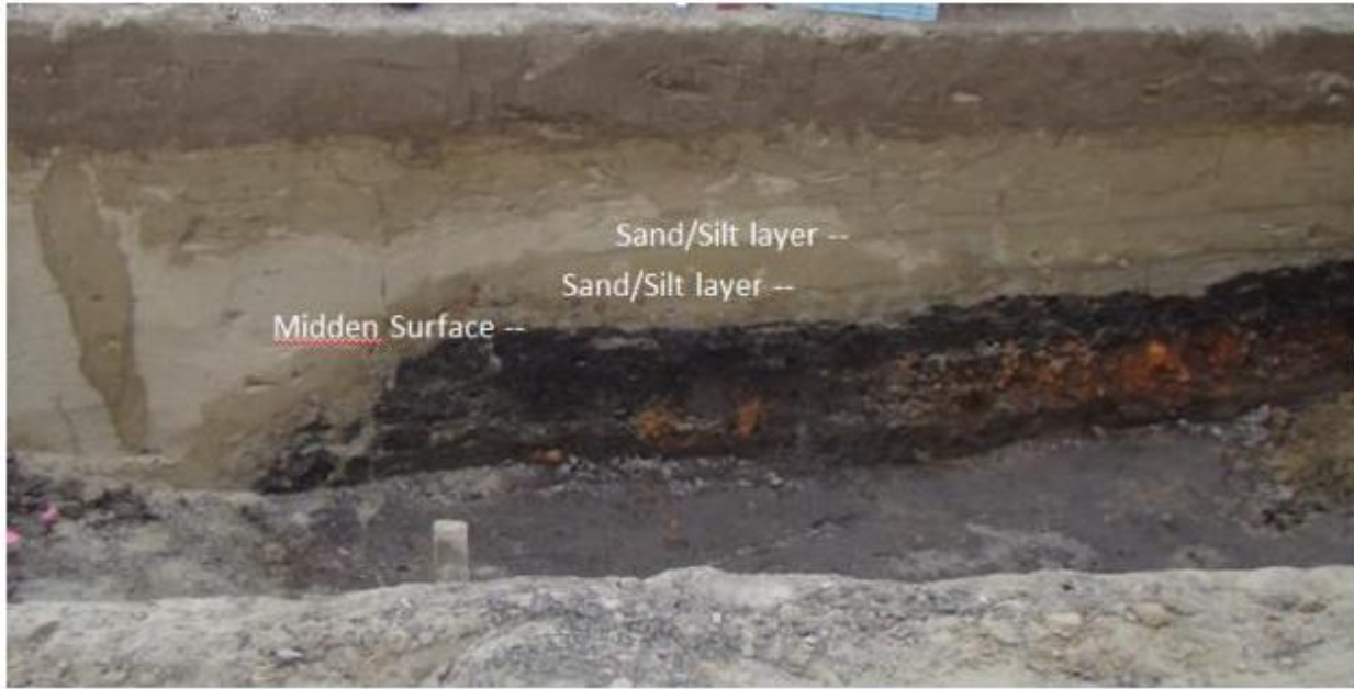
Figure 2-4: Sand dike (on left) with layers of sand and silt overlying the midden of an archaeological site (3MS106). The layering suggests at least two and likely three sand blows were extruded through the dike. The midden layer is now at a slight angle dipping toward the sand dike due to subsidence.
