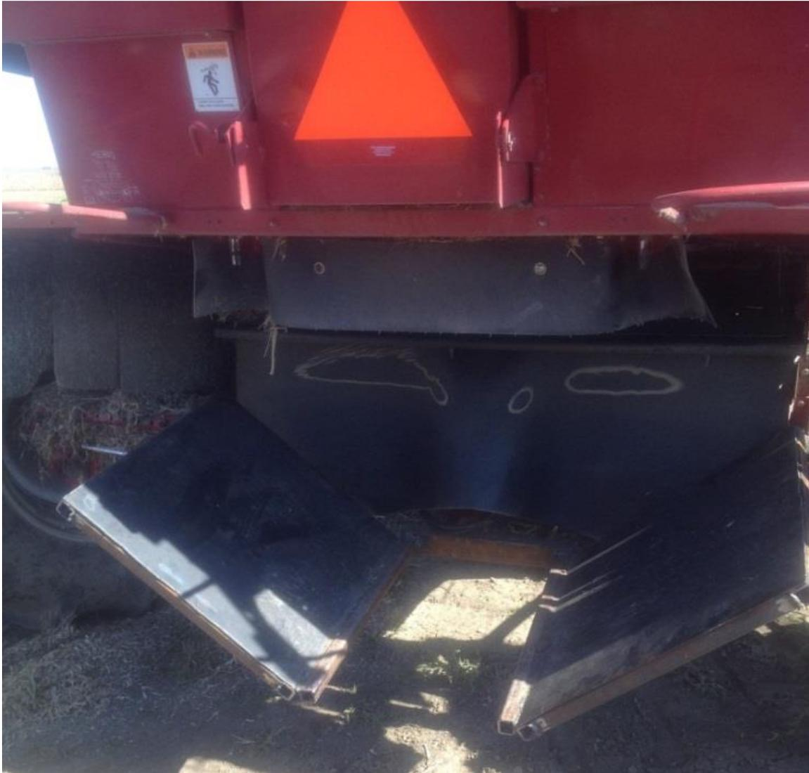
Figure 1.1. Narrow-windrow chute that funnels all harvest residues into a row for burning. The chute is attached to the rear of a Case 2388 combine in Keiser, Arkansas. (Photo by Author)
