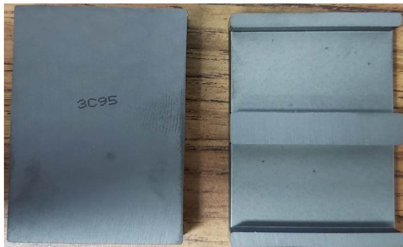
Fig. 10. Core halves - top and bottom view. [Image by author]
