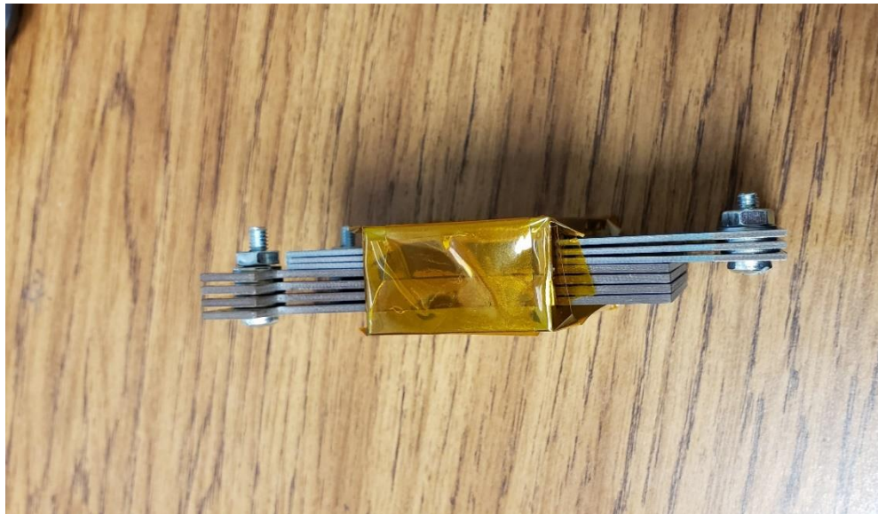
Fig. 13. Assembled planar transformer – side view. [Image by author]
