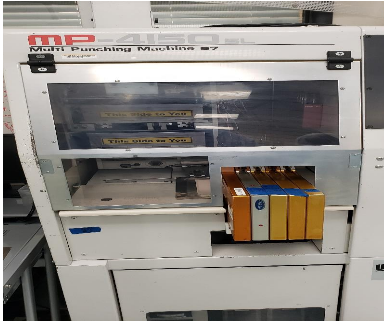
Fig. 20. Multi punching machine – MP-4150. [Image by author]
