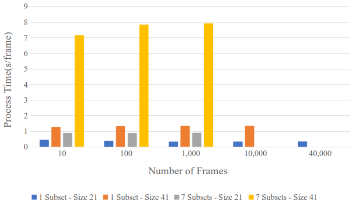
Figure 5.17: A bar graph that shows the total execution time per frame of the DICe hardware accelerator in reference to the number of frames, the number of subsets, and the size of the subsets
