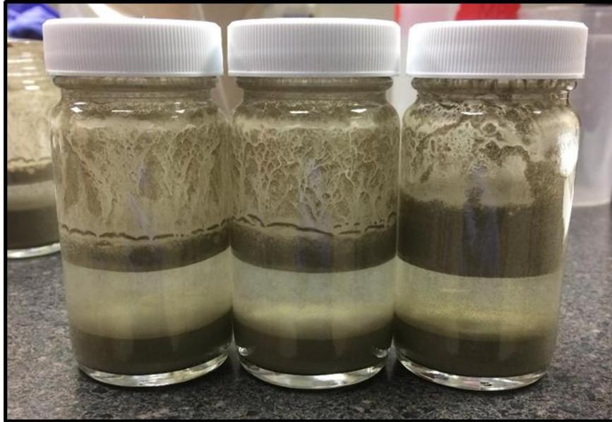
Figure 1. Comparison of Foam Index test jars at different AEA dosages. The two jars on the left have just reached the FI, while the far-right jar has greatly exceeded it, resulting in a large foam buildup.
