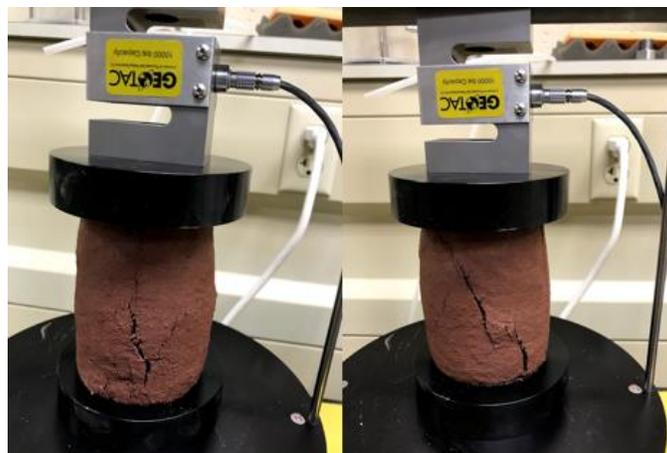
*Figure 21. Failure mechanism of the control group using 10% MC*
