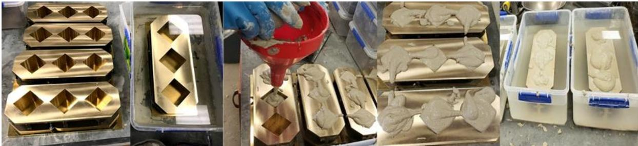
*Figure 2. Fresh mortar specimen casting set-up.*
