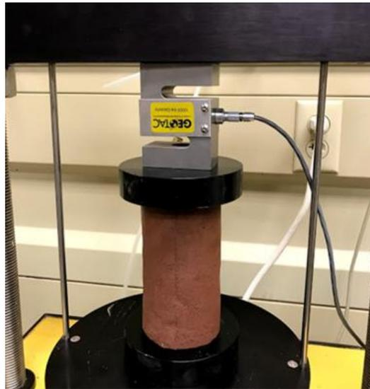
Figure 15. Set-up for a uniaxial unconfined compressive strength test.
