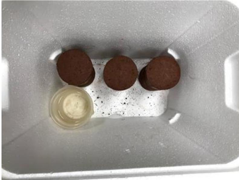
*Figure 14. Curing of the soil-cement specimens*
