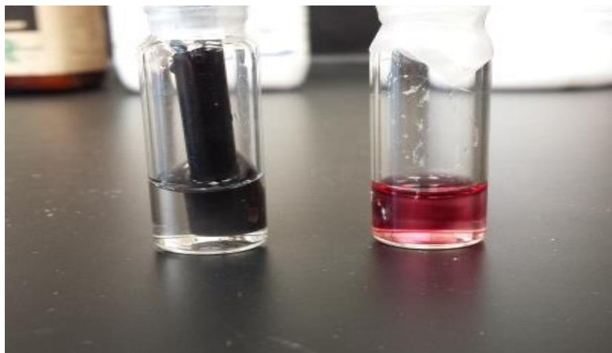
Figure 2.4 Colorimetric test results right after adding glucose: left vial- Ppy/GOx coated Pt electrode, right vial- known GOx solution.
