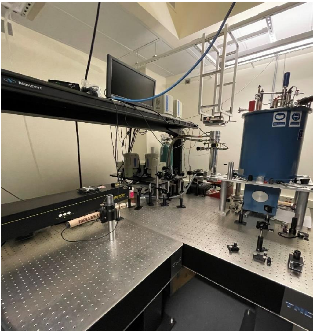
Figure 16. Photoluminescence (PL) measurement system.
