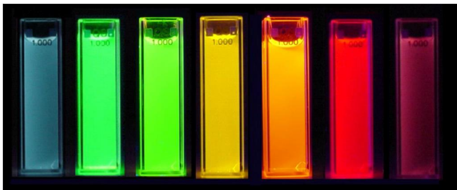
Figure 4 - CdSe QDs with sizes ranging from 2.5 nm (blue) to 6.5 nm (red) excited with the same 366 nm UV lamp
