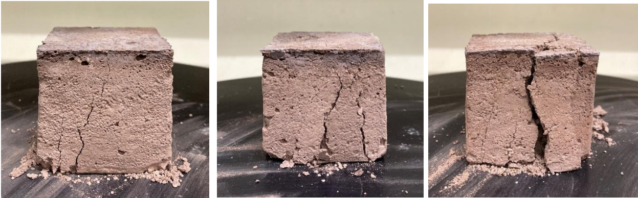
Figure 4.2.2 Failure behavior of cemented soil cubes.
