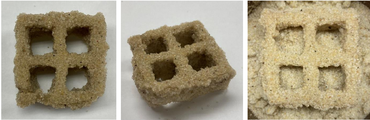
Figure 4.6.2 Cemented plantstalk layer, 100% Ottawa sand.
