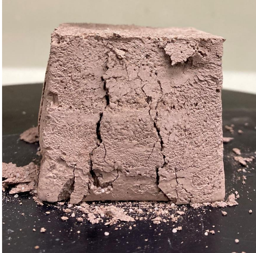
Figure 4.2.4 Failure behavior of an uncemented cube.
