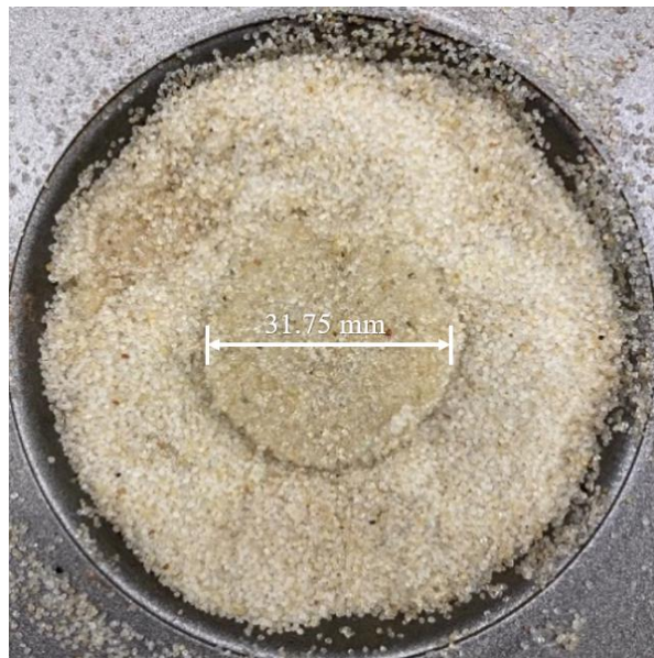
Figure 3.5.1 Circular layer of 100% Ottawa sand created using spray gels with the pump spray system.
