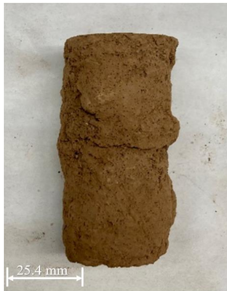
Figure 4.6.1 Cemented column, 50% sand 50% clay.
