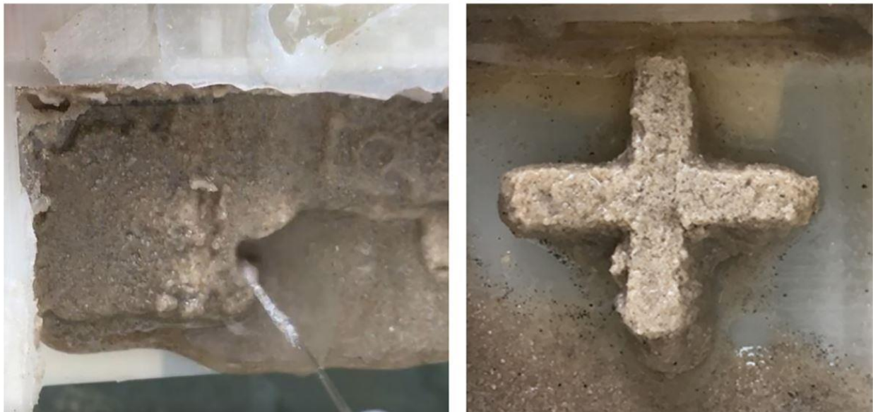
Figure 2.1.2.2.1.2 Results of selective soil treatment additive manufacturing (Nething et al., 2020).
