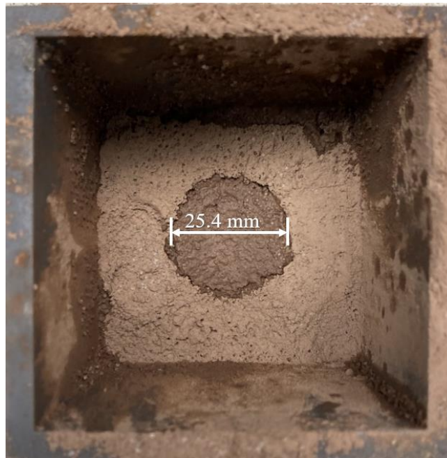
Figure 3.6.1 A layer in the column construction using a stencil.
