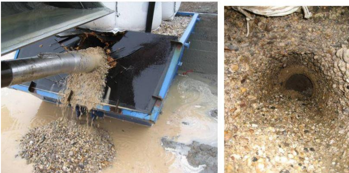
Figure 2.4.1.2 Borehole stability with gravel: (a) drilling into the prepared soil; and (b) the stable borehole (van Paassen, 2011).
