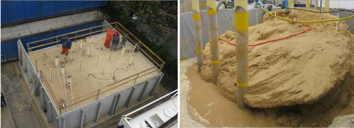
Figure 2.4.1.1 Large scale soil treatment using injection MICP: a) during treatment; and b) after treatment (van Paassen et al., 2009).
