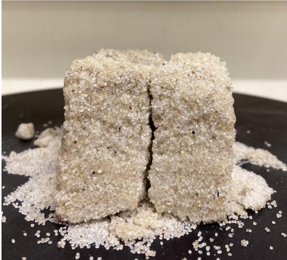
Figure 4.2.5 Failure behavior of a 100% Ottawa sand specimen.
