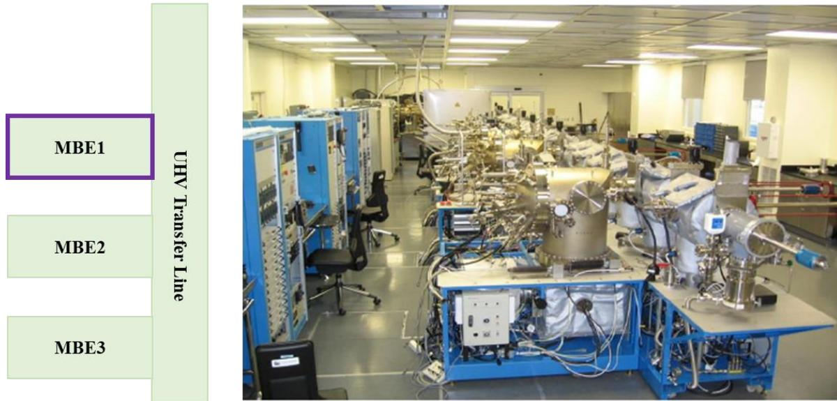
Figure 14: Three MBE chambers are connected by transfer line [55].
