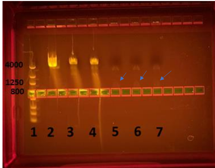
Figure.3: lane 1) standard DNA Ladder starting from 4000 bp to 100 bp. Lane 2) pET plasmid uncut 5443 bp. Lane 3,4) pET plasmid cleaved 5403 bp. 5,6,7) mlrA gene cleaved 1048 bp.
