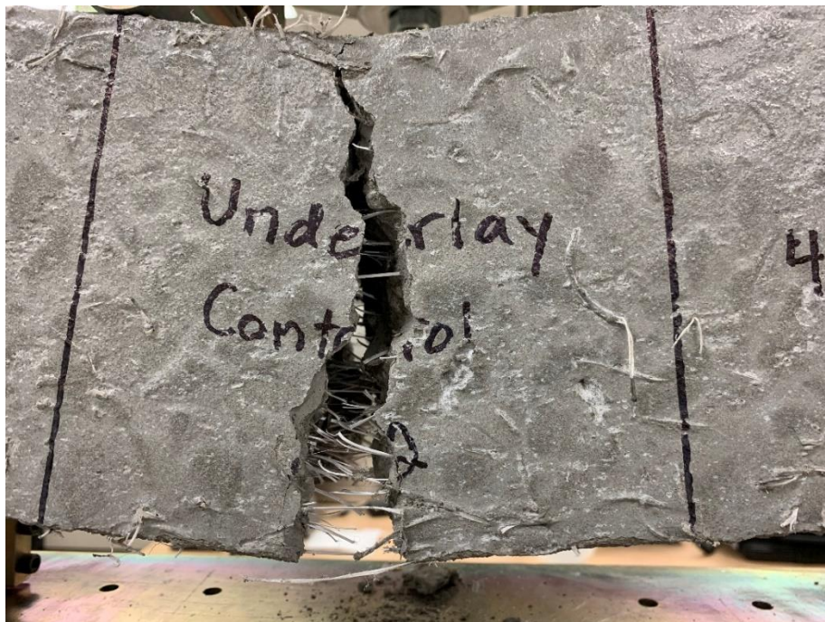
Figure 20. Fiber 2 FRC beam at end of test.
