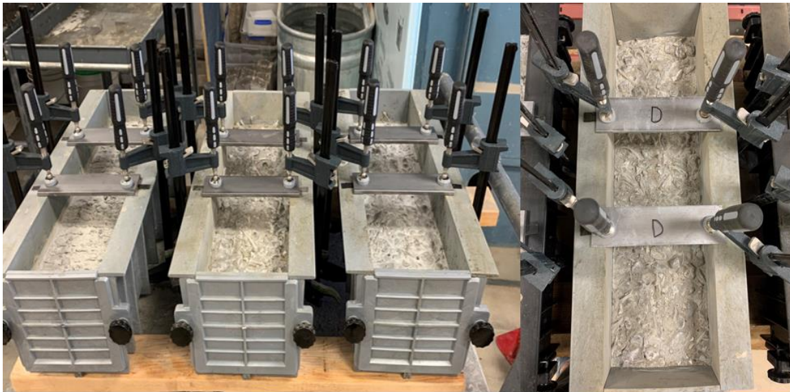
Figure 7. Formwork for hybrid beams.
