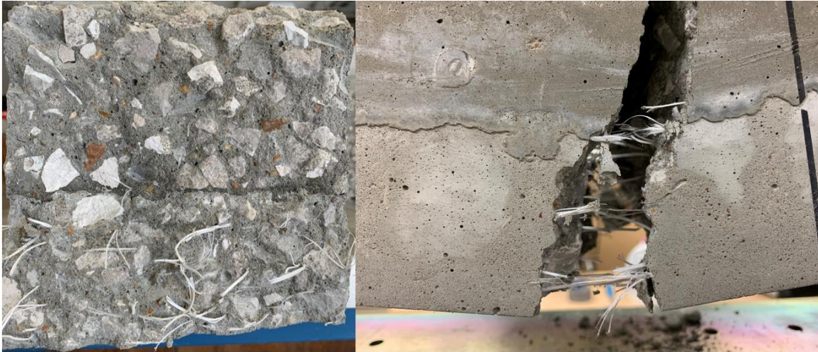
Figure 27. Example of hybrid cross section (left) and hybrid section at end of test (right).
