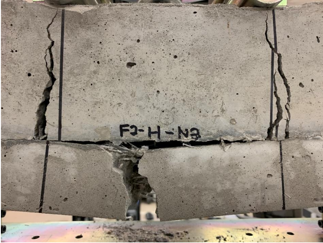
Figure 46. Worst case bond failure for hybrid beam with no surface preparation between layers at end of test.
