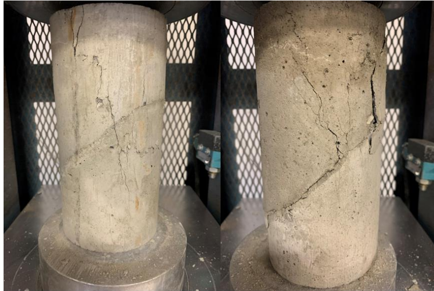
Figure 12. Failure in base materials (left) and shear failure at boundary interface (right).
