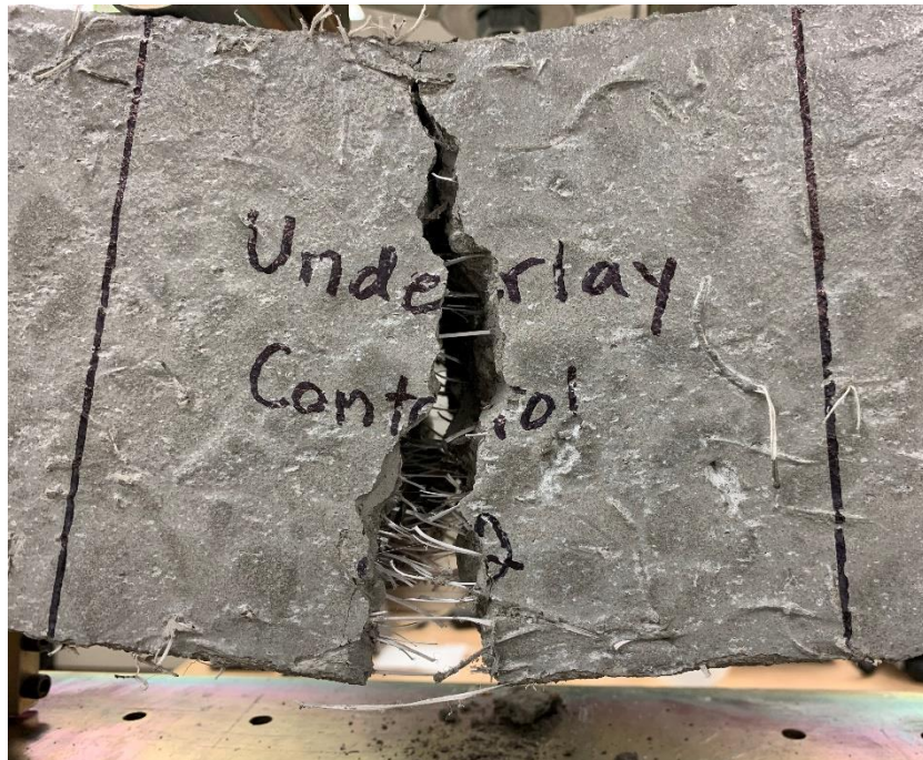
Figure 16. FRC beam at end of test.
