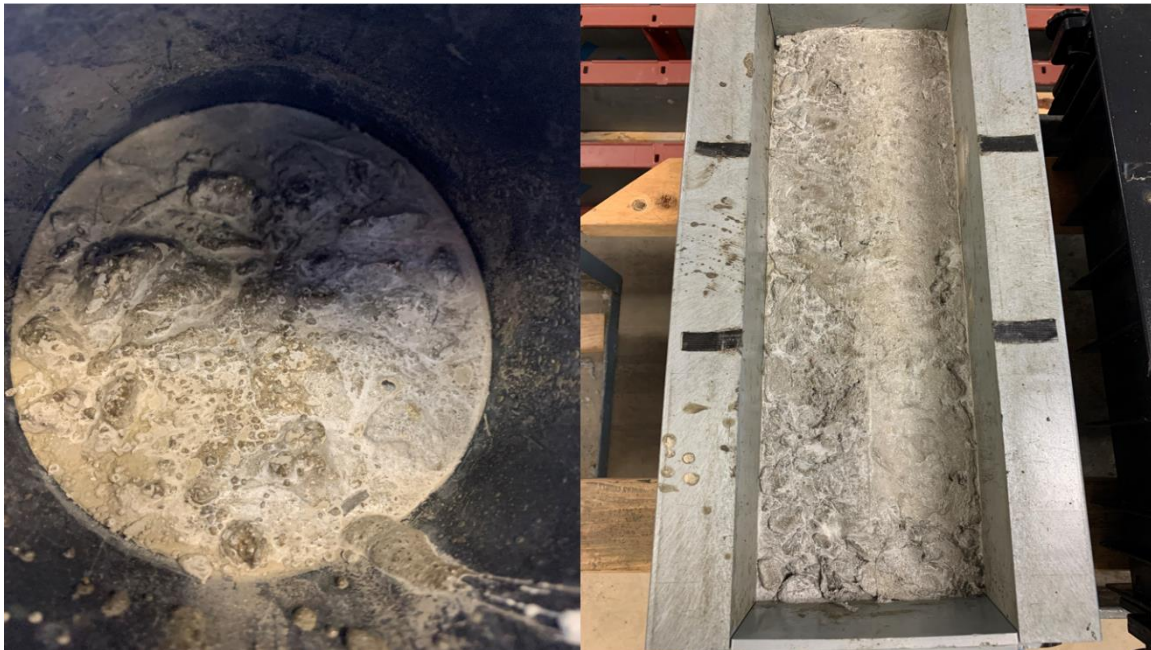
Figure 2. No surface preparation method for slant shear cylinders (left) and beams (right).
