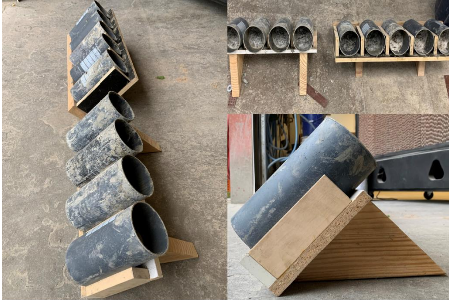
Figure 5. Formwork for slant-shear cylinders.
