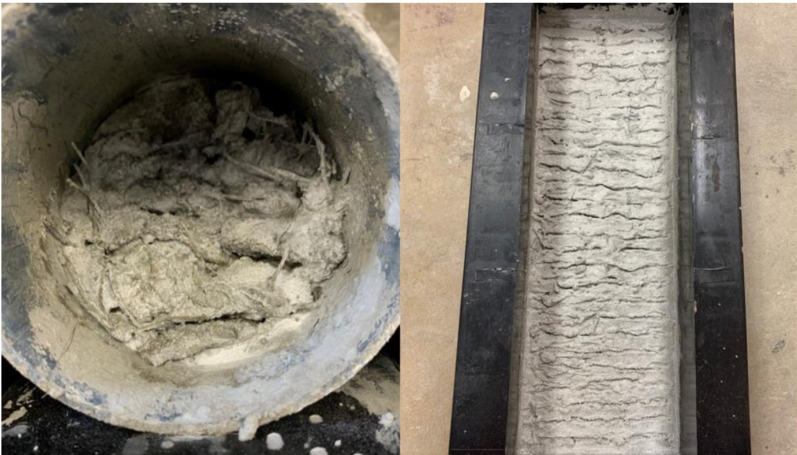
Figure 4. Example of tines surface preparation method for slant-shear cylinders (left) and beams (right).
