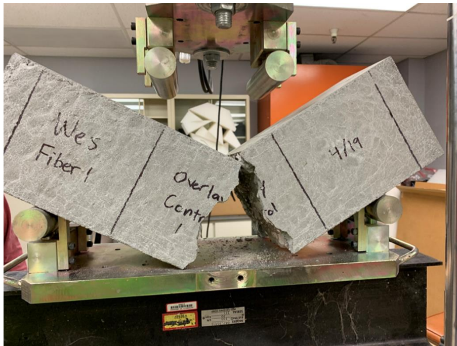
Figure 14. Typical failure of a PC beam.
