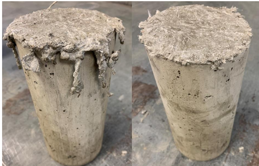
Figure 8. Fiber cylinder before trimming (left) and after trimming (right)
