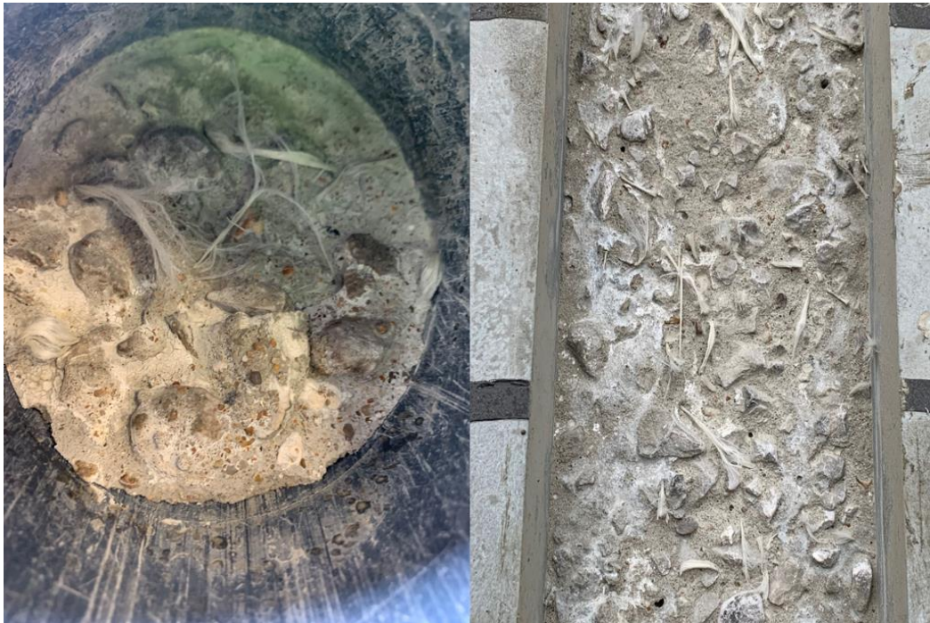
Figure 3. Example of DELVO surface preparation method for slant-shear cylinders (left) and beams (right).
