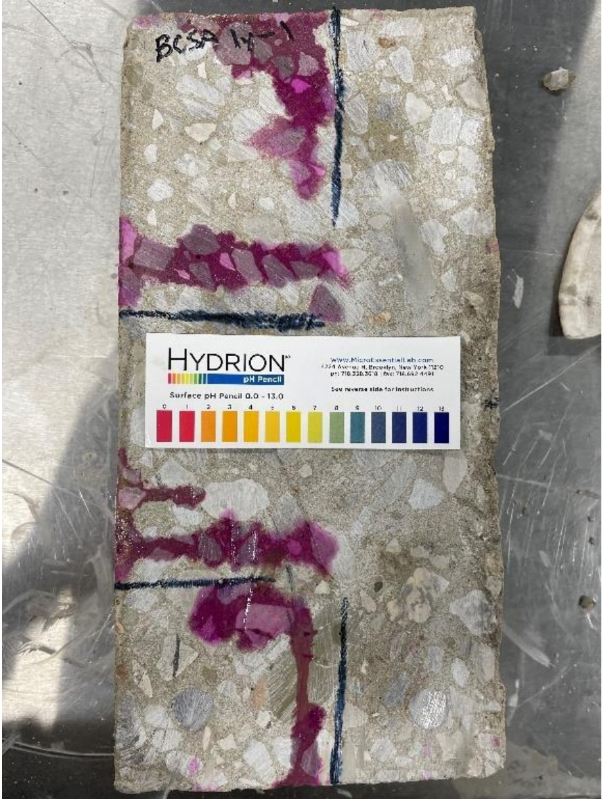
Figure 17. Carbonation test for BCSA 1y-1
