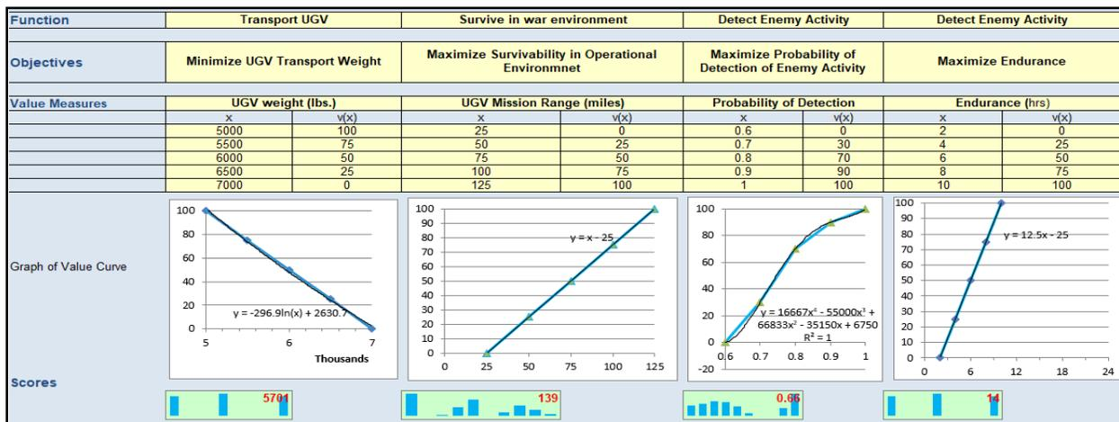
Figure 7. Preliminary Value Curves for a Notional UGV System
