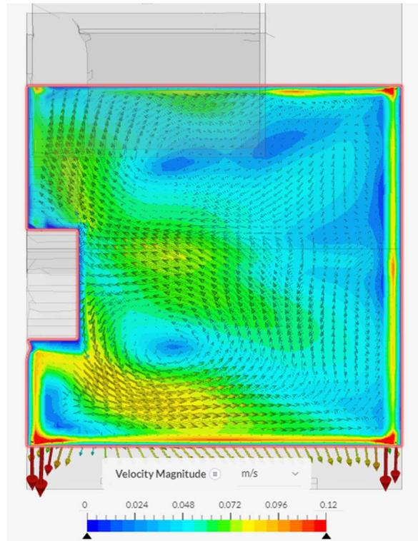
**Figure 29.** The circulation of cool air 1.1 meters above the floor at 600 seconds is shown.
