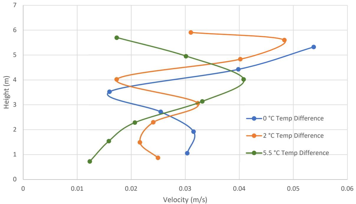
**Figure 46.** In the figure above, the air velocity, at 150 seconds, at varying heights for the 150-second cooling simulation is shown.
