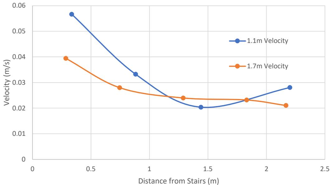
**Figure 64.** The air velocities at 1.1 and 1.7 meters for the 600-second heating simulation, with a 5.5 °C temperature difference, are shown.
