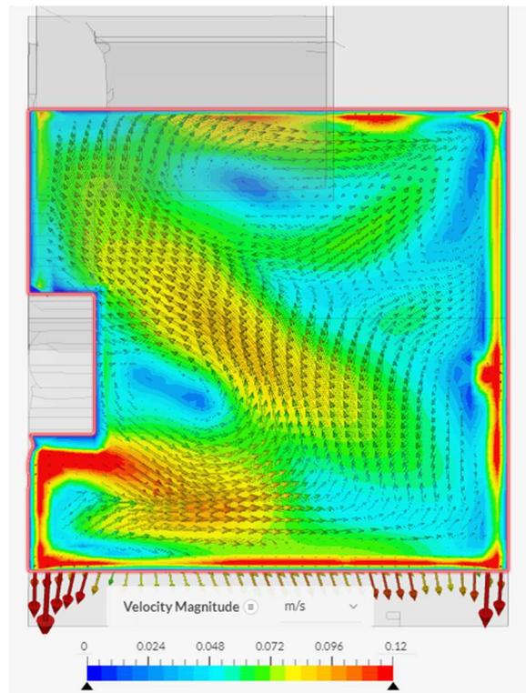
**Figure 28.** The circulation of cool air 1.1 meters above the floor at 150 seconds is shown.
