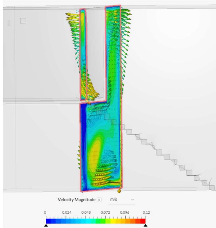
**Figure 26.** The air exchange through the doorway is shown at 150 seconds.
