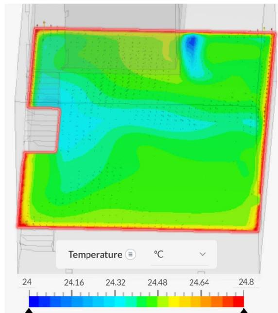
**Figure 19.** In the figure above, the temperature 1.7 meters above the floor at 100 seconds is shown.
