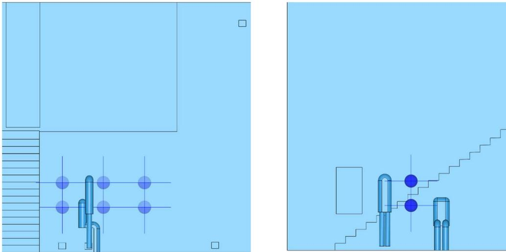
**Figure 45.** The heights of 1.1 and 1.7 meters above the ground are shown. The occupant to the left is standing, and the occupant to the right is sitting.
