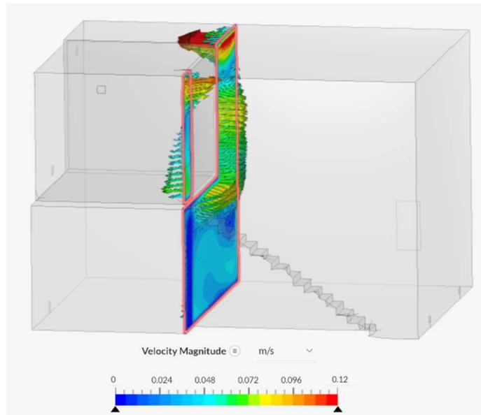
**Figure 12.** The air exchange through the doorway is shown at 150 seconds with the upper room 5.5 °C warmer.
