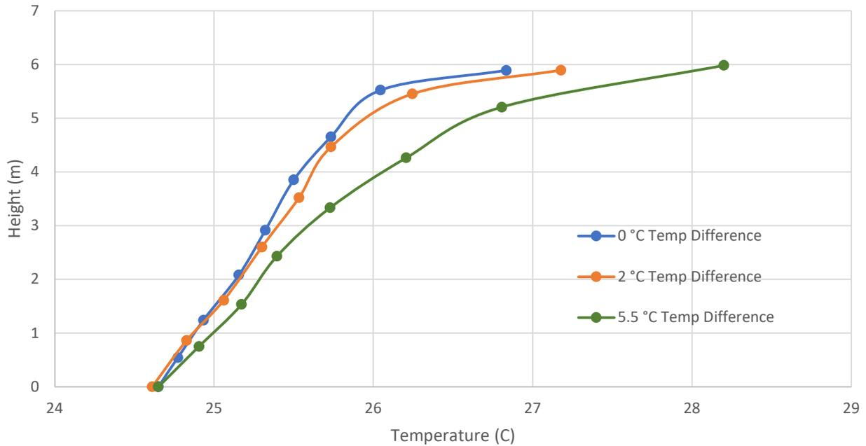
**Figure 49.** In the figure above, the air temperature, at 600 seconds, at varying heights for the 600-second cooling simulation is shown.
