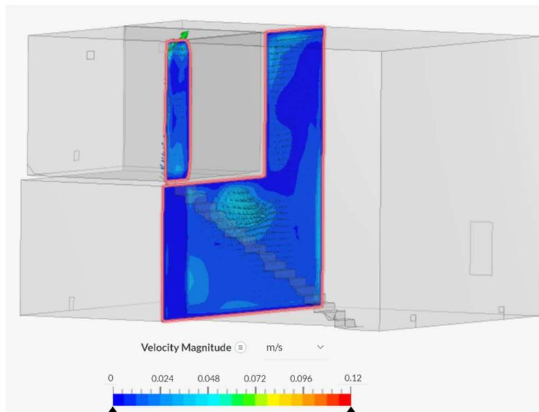
**Figure 13.** The air exchange through the doorway is shown at 600 seconds with the upper room 5.5 °C warmer.
