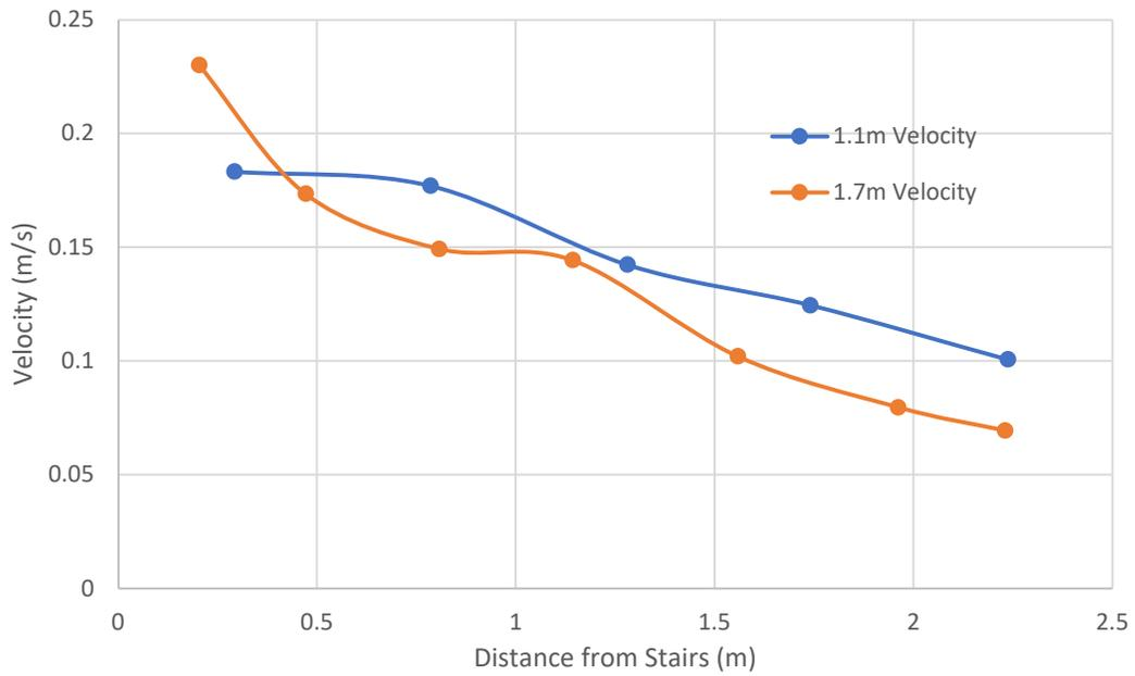
**Figure 60.** The air velocities at 1.1 and 1.7 meters for the 150-second heating simulation, with a 2 °C temperature difference, are shown.
