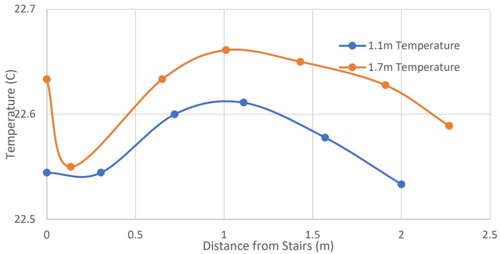
**Figure 58.** In the figure above, the air temperature, at 600 seconds, at 1.1 and 1.7 meters for the 600-second heating simulation, with a 5.5 °C temperature difference, is shown.
