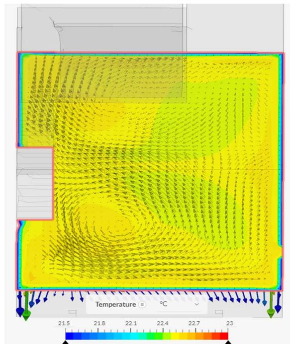
**Figure 39.** Air temperature 1.1 meters above the ground at 600 seconds with no initial temperature difference.
