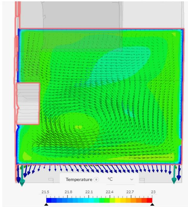
**Figure 40.** Air temperature 1.1 meters above the ground at 600 seconds with a 2 °C initial temperature difference.
