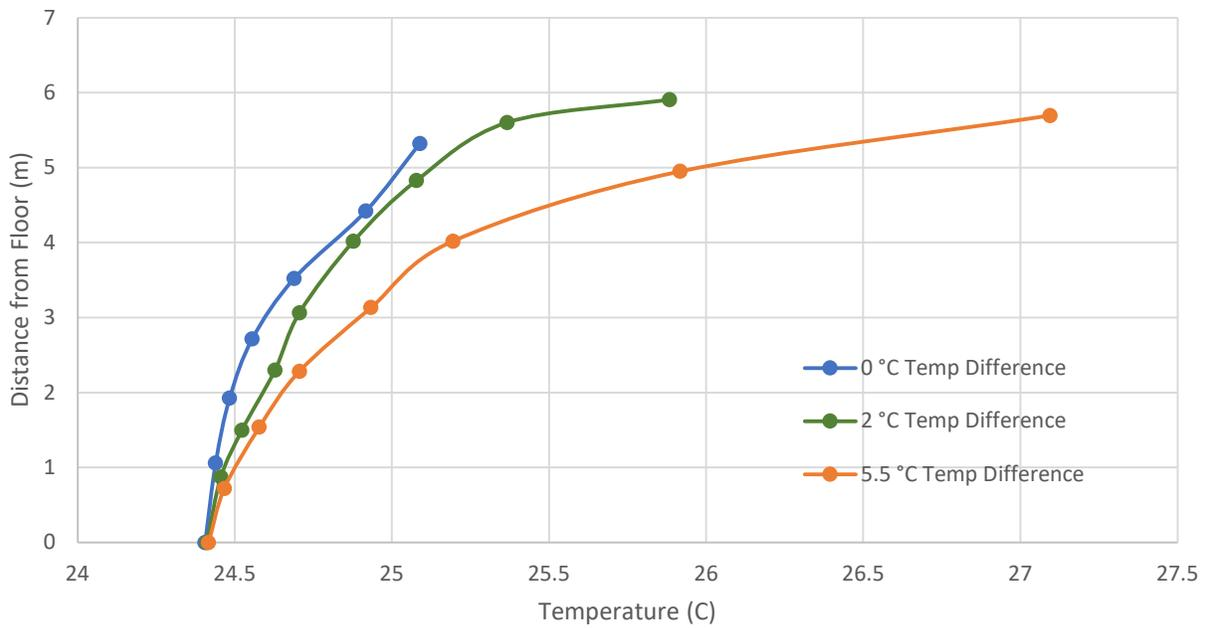
**Figure 48.** In the figure above, the air temperature, at 150 seconds, at varying heights for the 150-second cooling simulation is shown.
