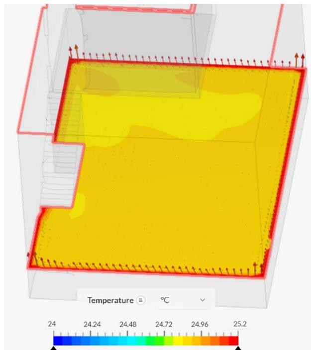
**Figure 16.** Air temperature 1.1 meters above the ground, at 600 seconds, with a temperature difference of 2 °C.
