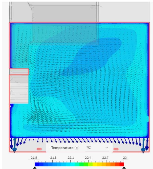
**Figure 41.** Air temperature 1.1 meters above the ground at 600 seconds with a 5.5 °C initial temperature difference.
