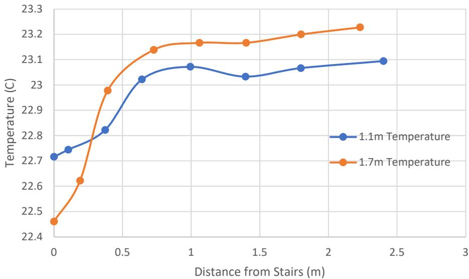
**Figure 55.** The air temperature at 150 seconds 1.1 and 1.7 meters for the 150-second heating simulation, with a 5.5 °C temperature difference, is shown.
