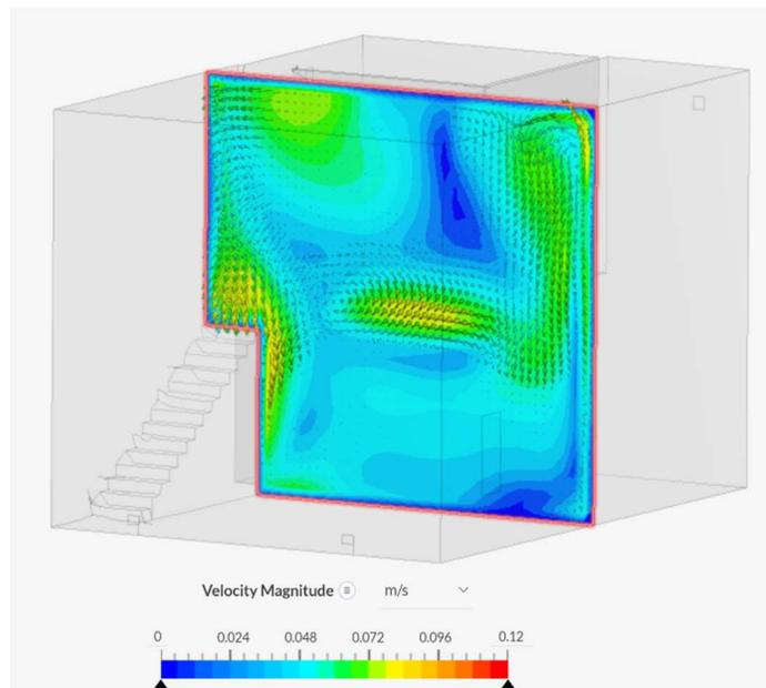
**Figure 6.** The airflow down and over the stairs is shown at 150-seconds.
