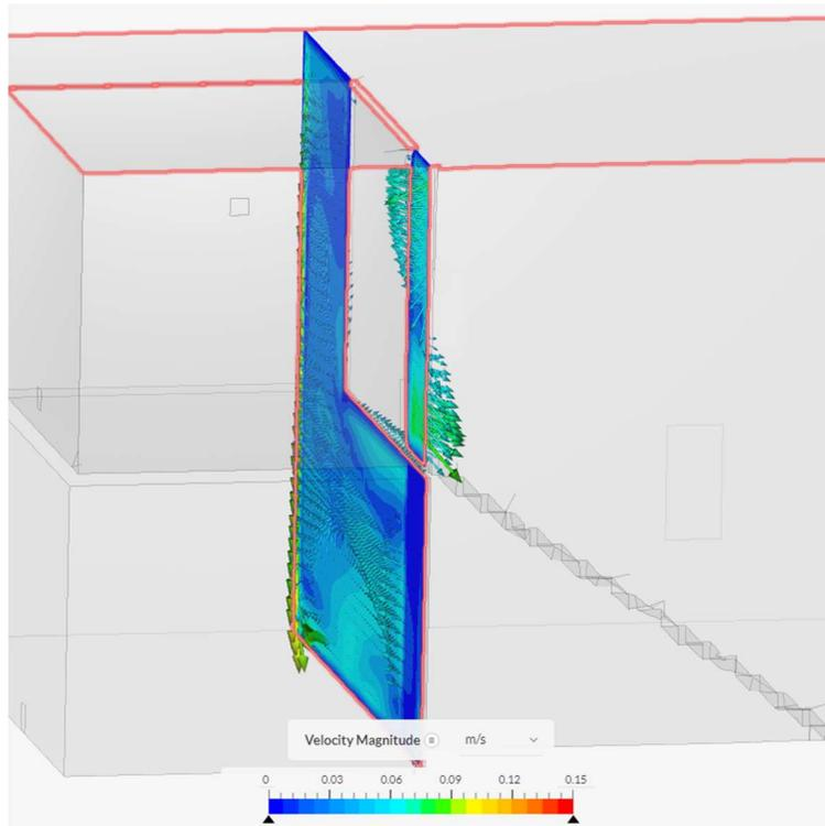
**Figure 33.** The air exchange through the doorway at 600 seconds is shown for a no initial temperature difference.
