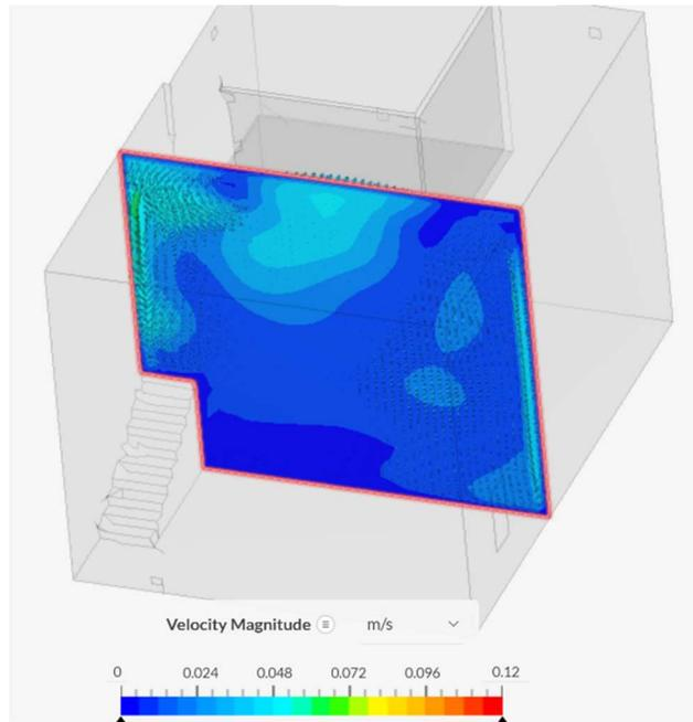
**Figure 9.** Warm air leaves the upper room and spreading across the ceiling at 600 seconds with the upper room starting at 2 °C warmer.
