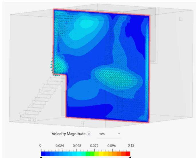
**Figure 7.** The airflow down and over the stairs is shown at 600 seconds.
