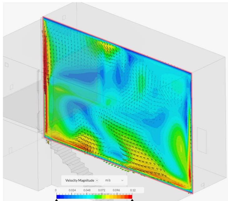
**Figure 24.** The air flows towards the staircase across the floor at 150 seconds.
