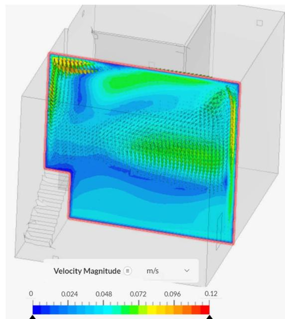
**Figure 8.** Warm air leaves the upper room and spreading across the ceiling at 150 seconds with the upper room starting at 2 °C warmer.
