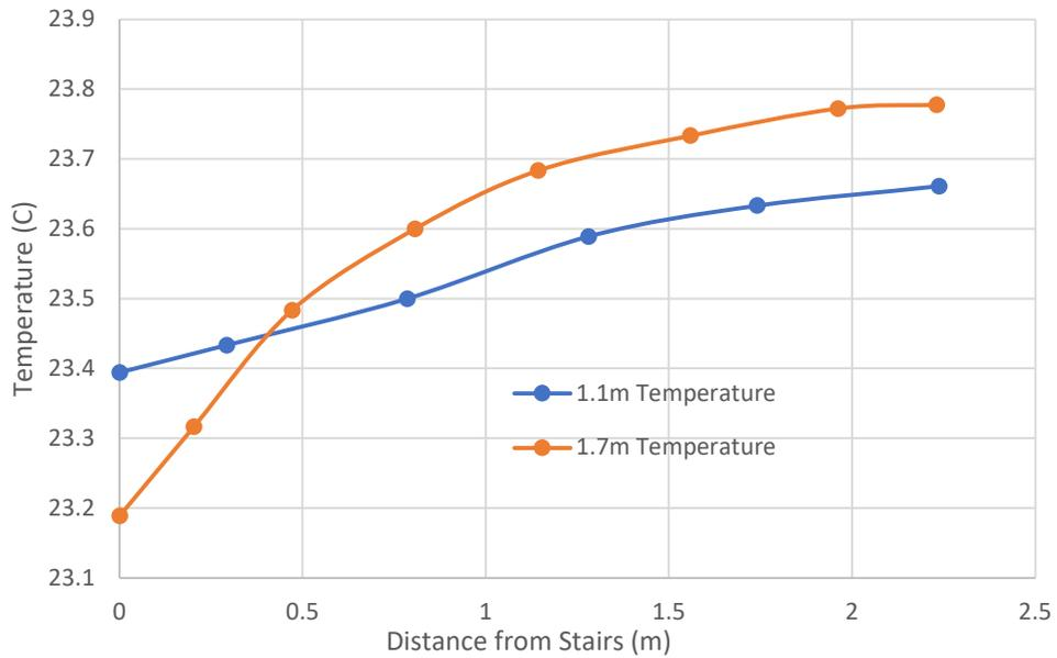
**Figure 54.** The air temperature at 1.1 and 1.7 meters for the 150-second heating simulation, with a 2 °C temperature difference, is shown.
