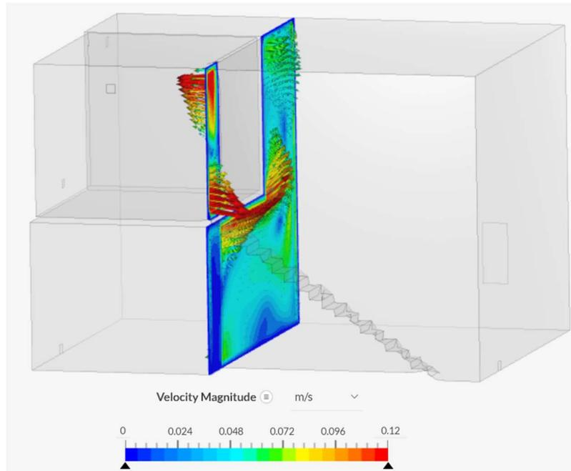
**Figure 20.** The air exchange through the doorway is shown at a time of 100 seconds.
