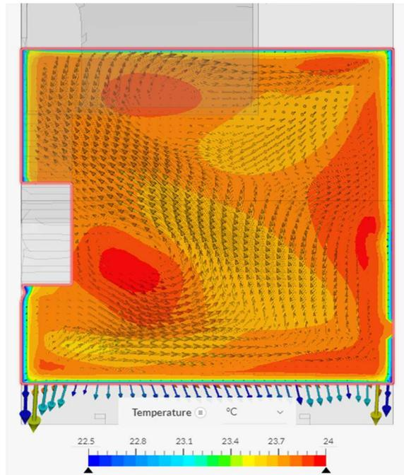
**Figure 36.** Air temperature 1.1 meters above the ground at 150 seconds with no initial temperature difference.
