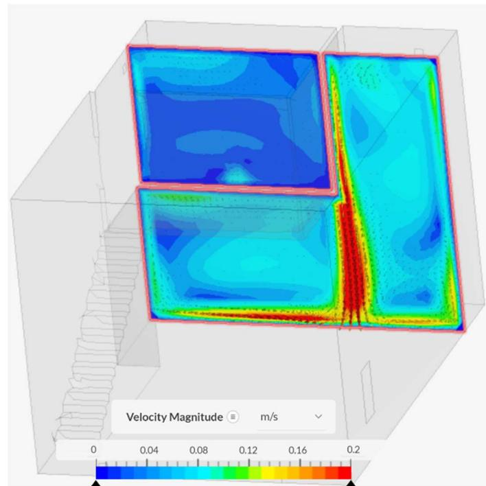
**Figure 18.** The air from the main inlet on the back wall comes into the building and crashes down into the main area at the 100 second mark.
