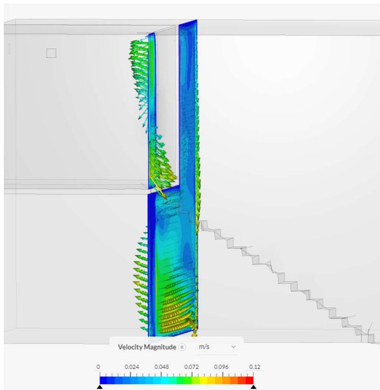
**Figure 27.** The air exchange through the doorway is shown at 600 seconds.
