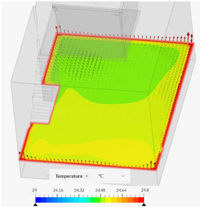
**Figure 15.** Air temperature 1.1 meters above the ground, at 150 seconds, with a temperature difference of 5.5 °C.
