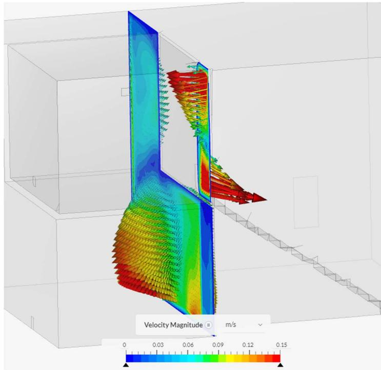
**Figure 31.** The air exchange through the doorway at 150 seconds is shown for a 2 °C initial temperature difference.
