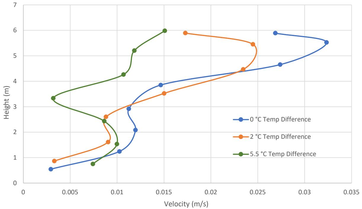
**Figure 47.** In the figure above, the air velocity, at 600 seconds, at varying heights for the 600-second cooling simulation is shown.
