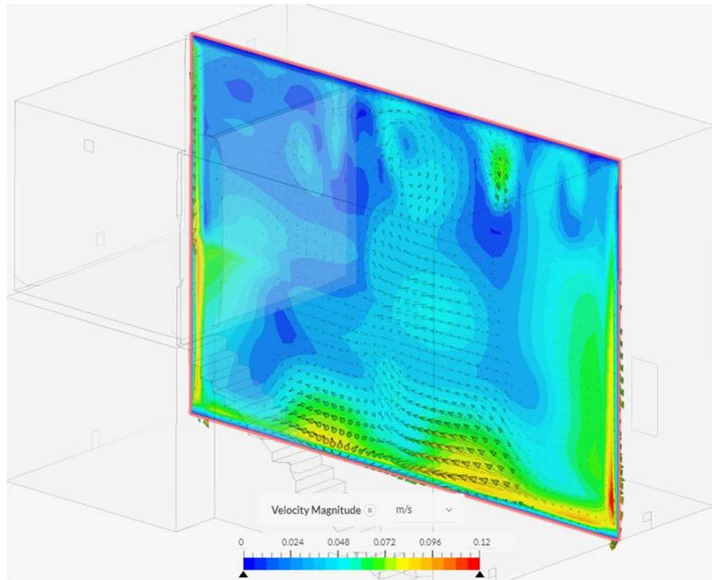
**Figure 25.** The air flows towards the staircase across the floor at 600 seconds.
