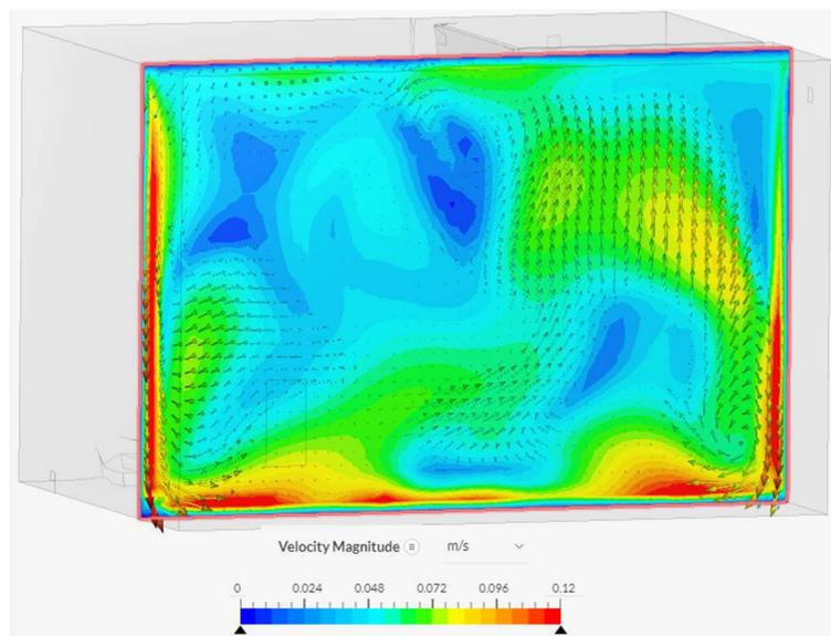
**Figure 22.** The natural circulation of air near the walls is shown at 150 seconds.
