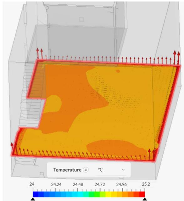
**Figure 17.** Air temperature 1.1 meters above the ground, at 600 seconds, with a temperature difference of 5.5 °C.
