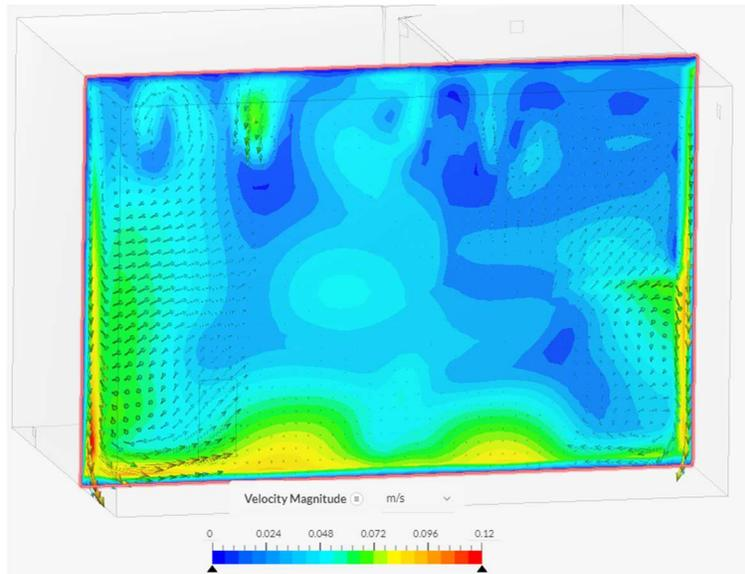
**Figure 23.** The natural circulation of air near the walls is shown at 600 seconds.
