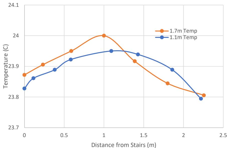
**Figure 53.** The air temperature, at 150 seconds, at 1.1 and 1.7 meters for the 150-second heating simulation is shown.
