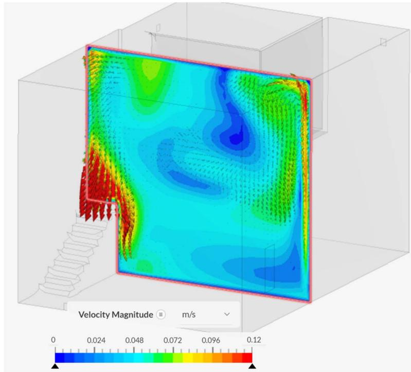
**Figure 21.** In the figure above, the air is shown to move down the stair and partly spill over the side into the main area at 100 seconds.
