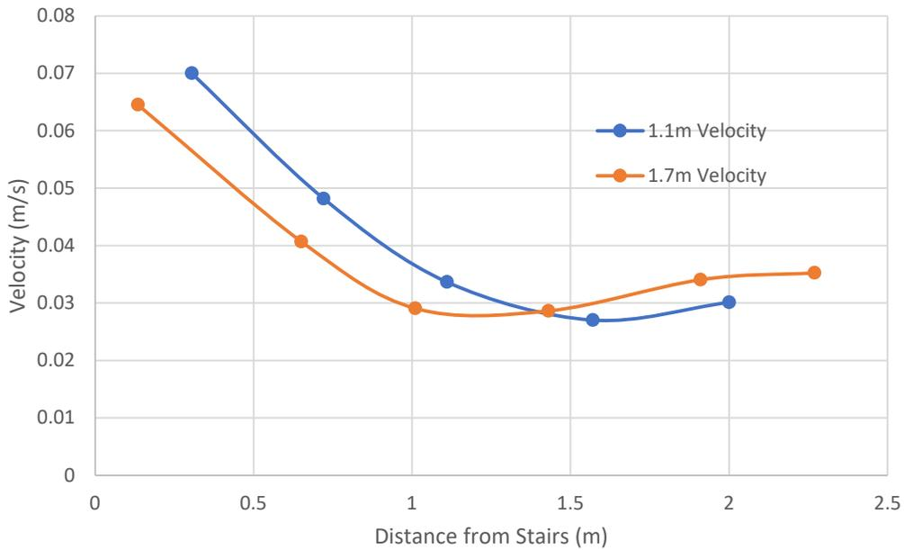
**Figure 63.** The air velocities at 1.1 and 1.7 meters at 600 seconds in the heating simulation, with a 2 °C temperature difference, are shown.
