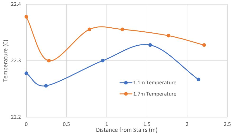
**Figure 57.** The air temperature at 1.1 and 1.7 meters for the 600-second heating simulation, with a 2 °C temperature difference, is shown.
