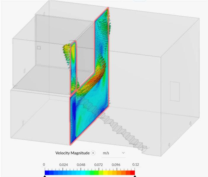
**Figure 4.** The air exchange through the doorway at 150 seconds is shown.
