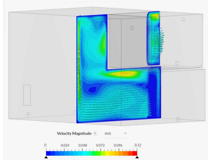
**Figure 10.** The air exchange through the doorway, from a rear view, is shown at 150 seconds with the upper room 2 °C warmer.
