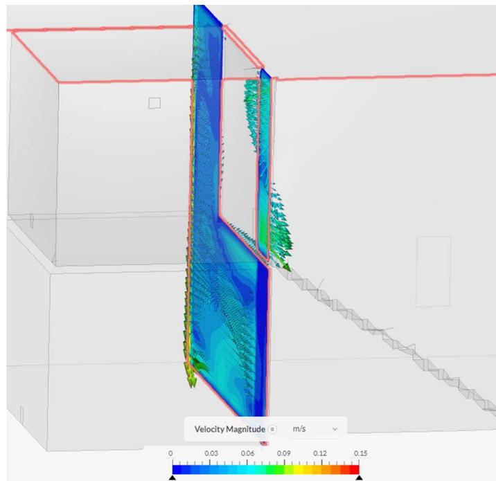
**Figure 34.** The air exchange through the doorway at 600 seconds is shown for a 2 °C initial temperature difference.
