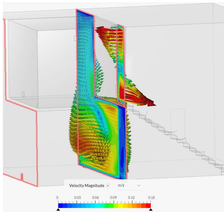
**Figure 32.** The air exchange through the doorway at 150 seconds is shown for a 5.5 °C initial temperature difference
