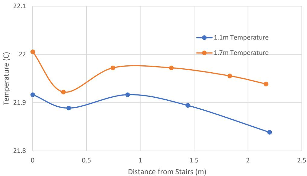
**Figure 56.** In the figure above, the air temperature, at 600 seconds, at 1.1 and 1.7 meters for the 600-second heating simulation is shown.
