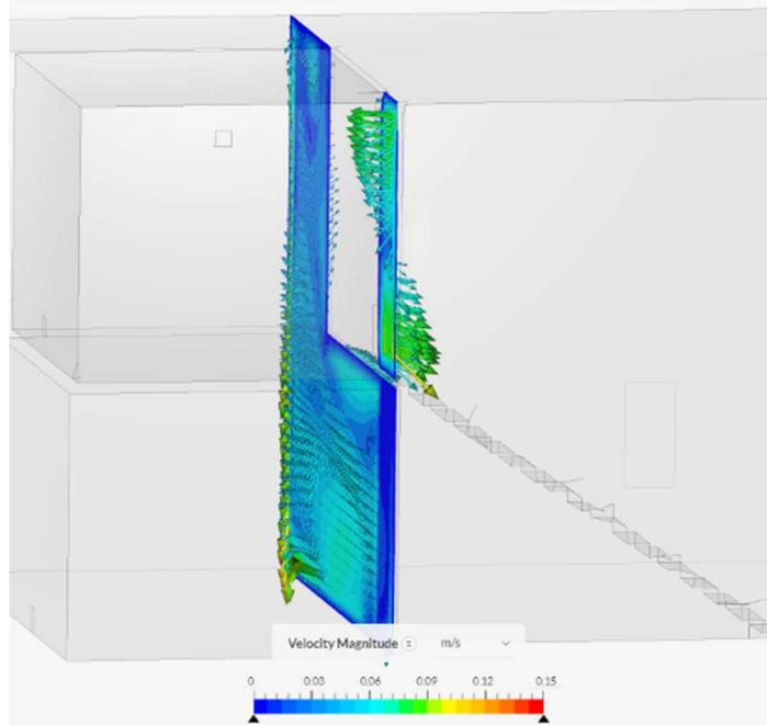
**Figure 35.** The air exchange through the doorway at 600 seconds is shown for a 5.5 °C initial temperature difference.
