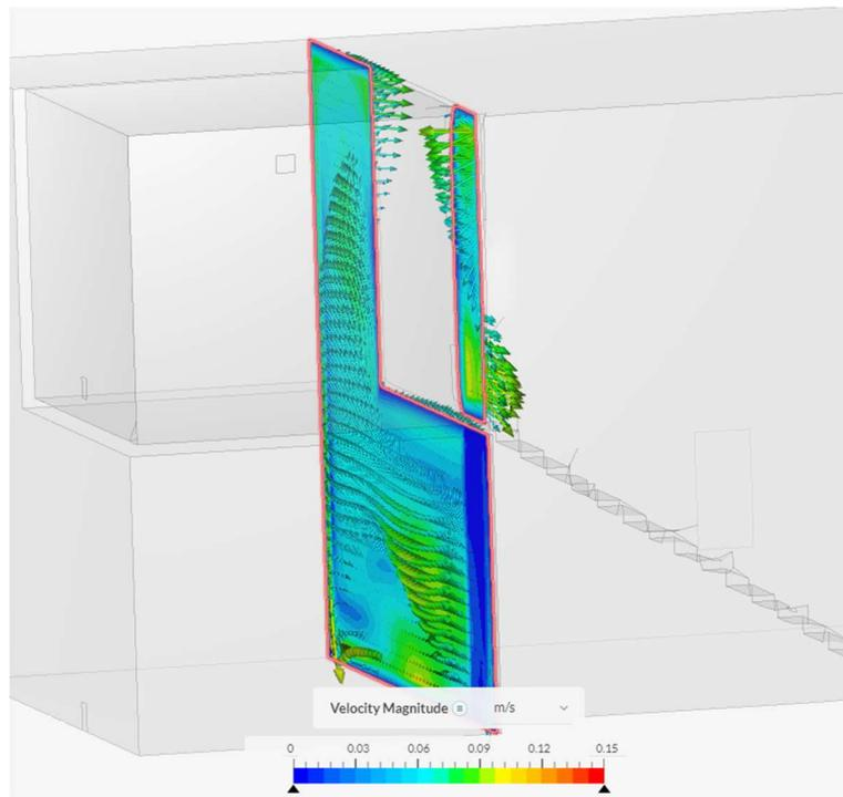
**Figure 30.** The air exchange through the doorway at 150 seconds is shown for no initial temperature difference.
