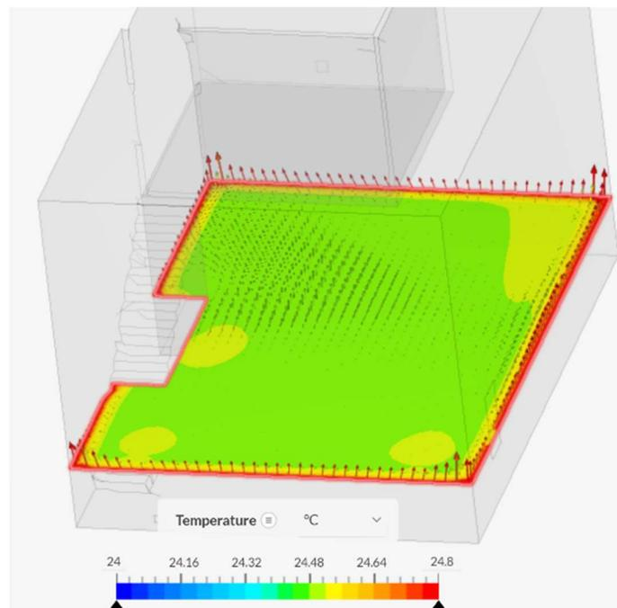
**Figure 14.** Air temperature 1.1 meters above the ground, at 150 seconds, with a temperature difference of 2 °C.
