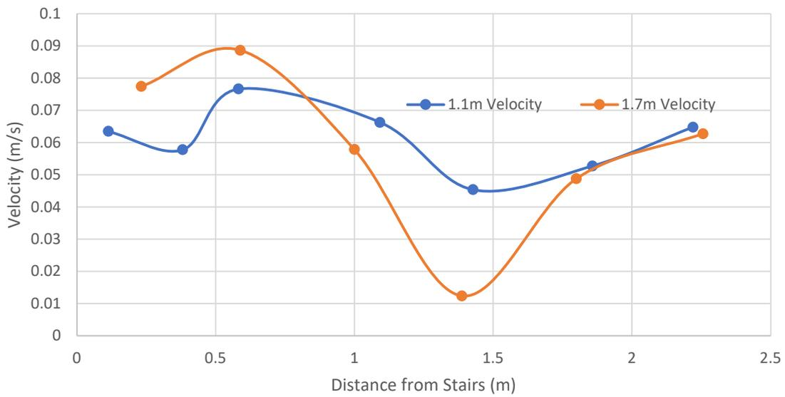
**Figure 59.** The air velocities at 1.1 and 1.7 meters for the 150-second heating simulation are shown.
