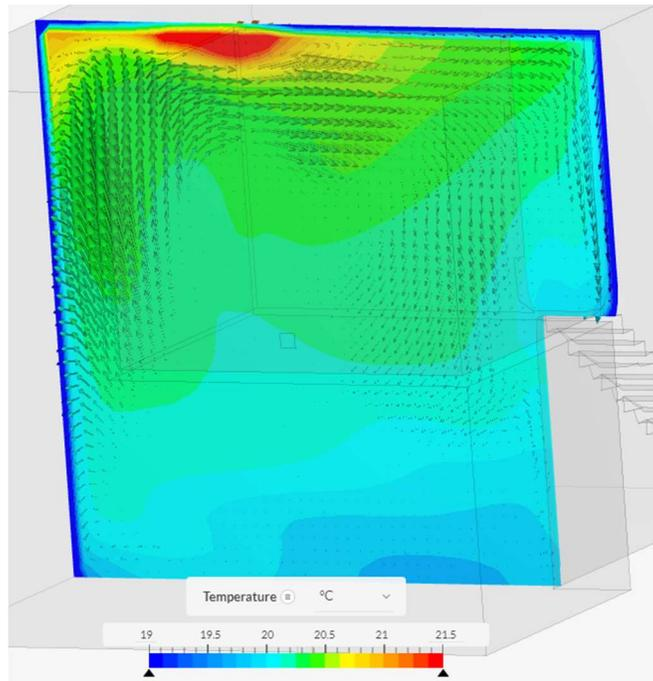
**Figure 43.** From the rear view of the building at 100 seconds, the air from the upper portion of the main area wraps around the doorway and enters the room.
