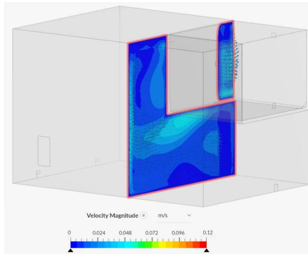
**Figure 11.** The air exchange through the doorway, from a rear view, is shown at 600 seconds with the upper room 2 °C warmer.
