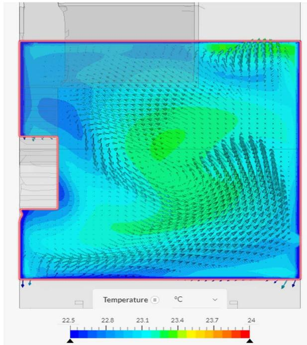
**Figure 38.** Air temperature 1.1 meters above the ground at 150 seconds with a 5.5 °C initial temperature difference.
