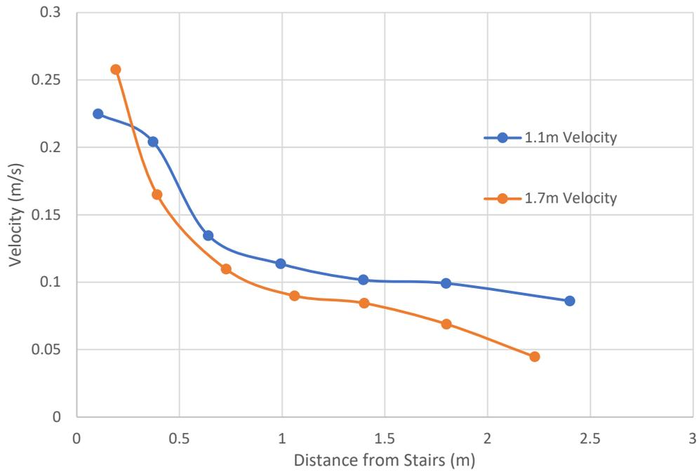
**Figure 61.** The air velocities at 1.1 and 1.7 meters at 150 seconds in the heating simulation, with a 5.5 °C temperature difference, are shown.
