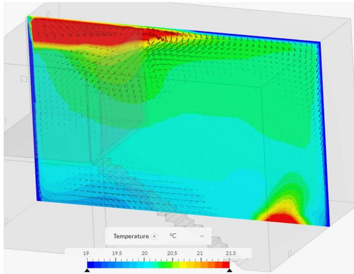
**Figure 42.** In this view from the left side of the building at 100 seconds, the inlet air is seen moving towards the left wall and wrapping around the outside of the room wall.
