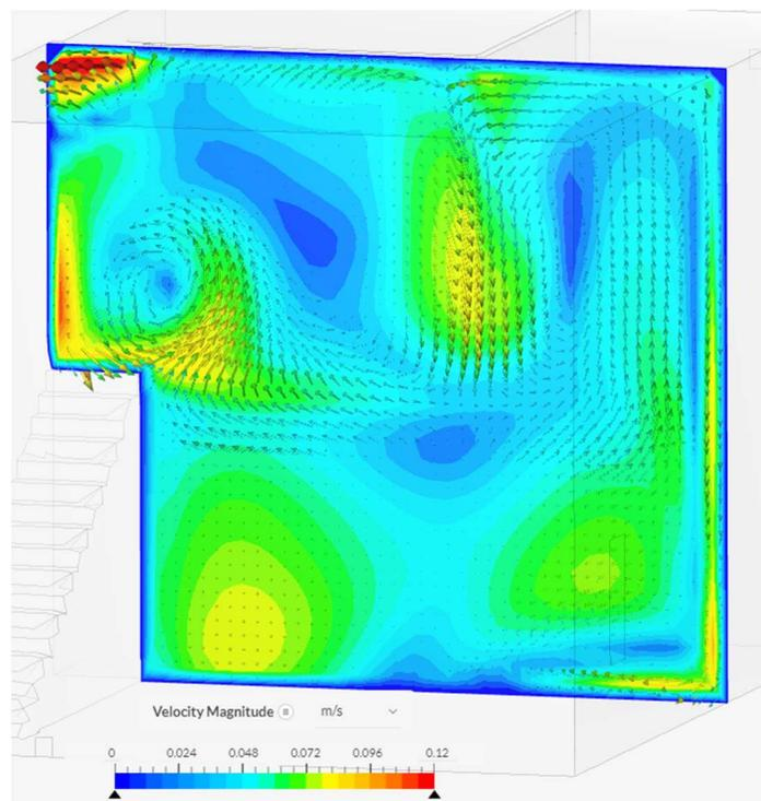
**Figure 44.** The circulation of air outside of the doorway is shown at 100 seconds the top of the stairs.
