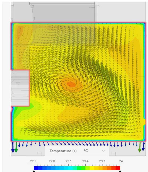
**Figure 37.** Air temperature 1.1 meters above the ground at 150 seconds with a 2 °C initial temperature difference.
