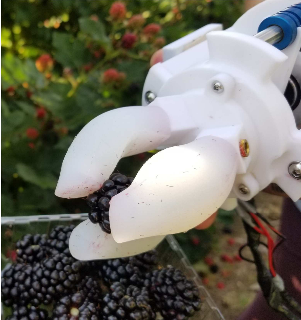
Fig. 2. Soft robotic gripper prototype developed at the University of Arkansas grasping a fresh-market blackberry (Arkansas, 2021)
