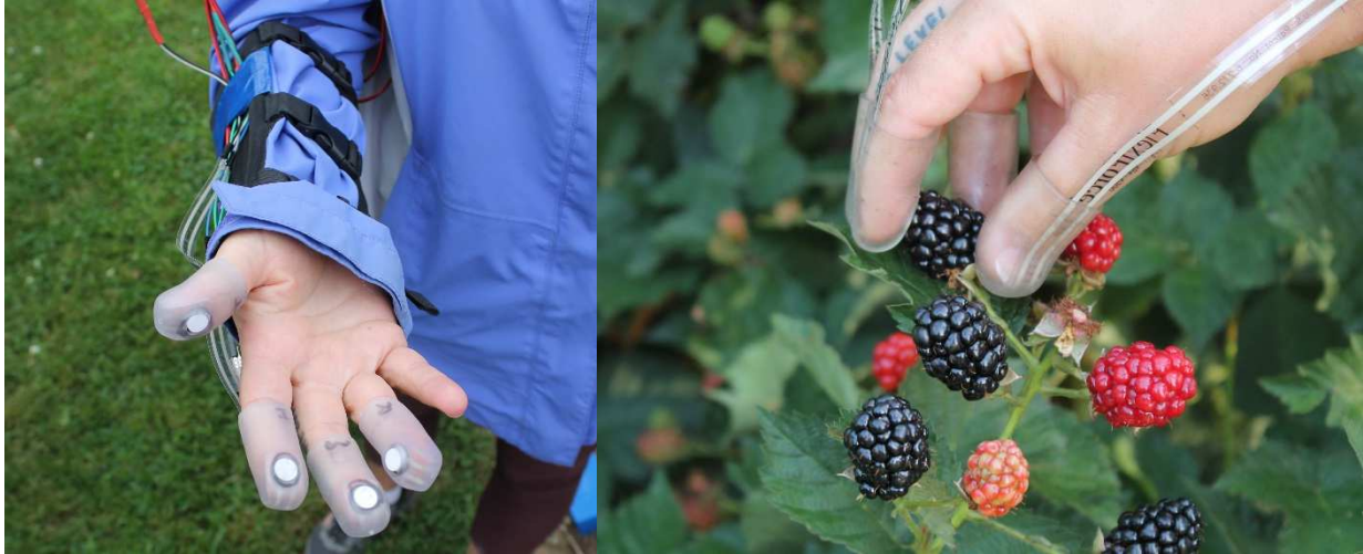
Fig. 1. Custom-made force sensing apparatus developed at the University of Arkansas with sensors on the thumb and three fingers (left) placed on the hand for harvesting (right) fresh-market blackberries (Arkansas, 2020).
