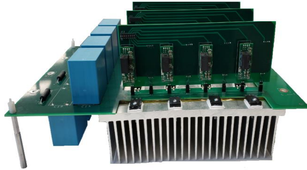
Figure 2-12 Experimental prototype picture of a 10-kW hybrid Si/SiC switch based ANPC inverter.
