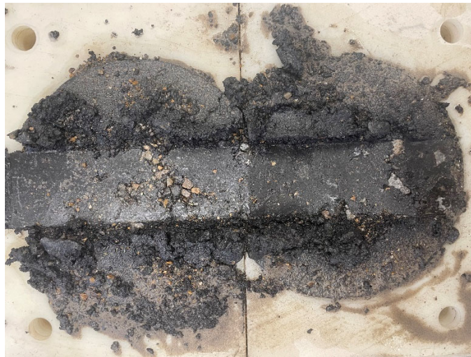
Figure 8. Hamburg Wheel Track Testing specimen with visible evidence stripping
