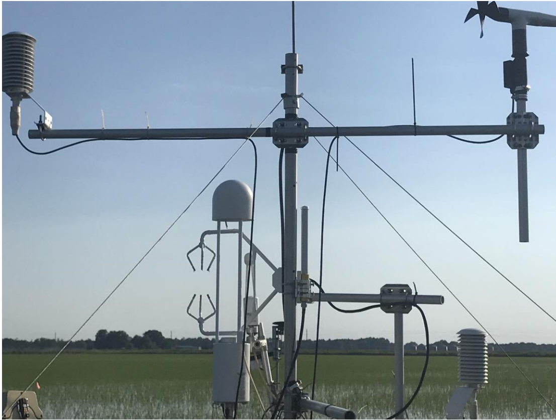
Figure 2: Eddy covariance and meteorological instrumentation on the study site (South Field) with measuring equipment, taken summer 2021. Photo by Dawson Oakley.
