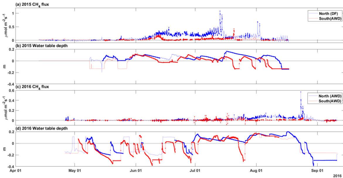
Figure 5: (a) Interpolated, gap-filled daily \text{CH}_4 flux for 2015. (b) Water level measurements for 2015. (c) Interpolated, gap-filled daily \text{CH}_4 flux for 2016. (d) Water level measurements for 2016. The North field in 2015 was managed with DF while the South field in 2015 and both fields in 2016 were managed with AWD. All fields were dry seeded. Note the difference in scale between the y axes in (a) and (c). Darker points indicate observed data while paler lines indicate modelled data.
