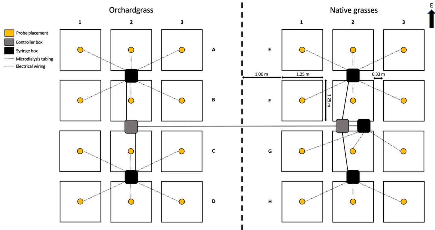
**Figure 2.** Experimental setup in the field. The approximate center of each plot ( $n = 12$  in each grass type) was implanted with a microdialysis probe. The controllers and syringe pumps were housed in weighted Styrofoam boxes and all microdialysis tubing and electrical wiring was protected using CVPC pipes.
