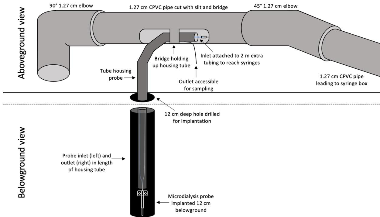
**Figure 3.** The protective bridge constructed to protect the probe outlet and tubing connection from warping or kinking.
