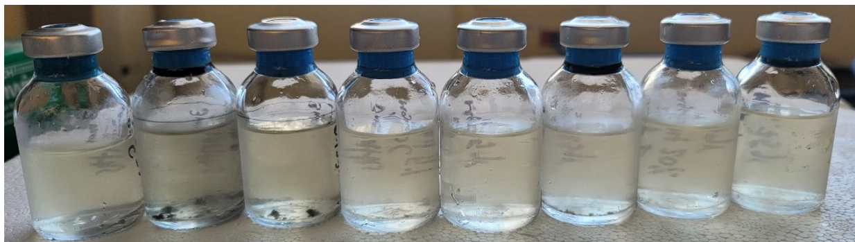
Figure 33. Cultures incubated at -10 °C for 90 days and supplemented with MgSO 4 . From left to right: Growth negative control, 0.35 wt%, 1 wt%, 5 wt%, 10 wt%, 15 wt%, 20 wt%, and 25 wt% supplementations with MgSO 4 .
