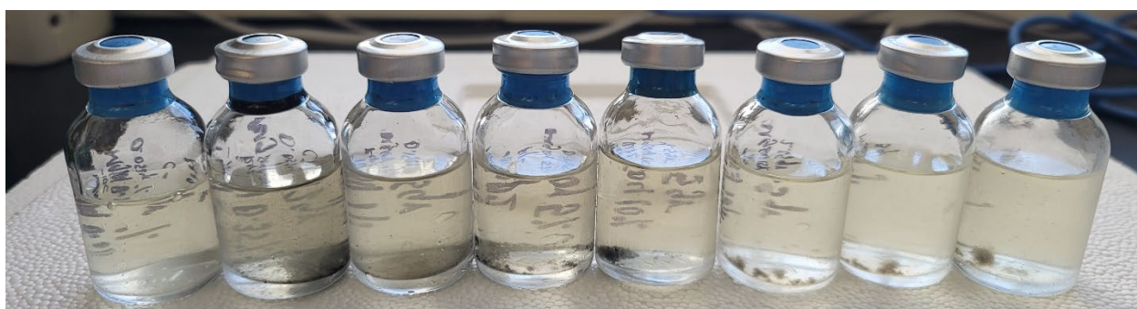
Figure 32. Cultures incubated at -10 °C for 30 days and supplemented with MgSO 4 . From left to right: Growth negative control, 0.35 wt%, 1 wt%, 5 wt%, 10 wt%, 15 wt%, 20 wt%, and 25 wt% supplementations with MgSO 4 .
