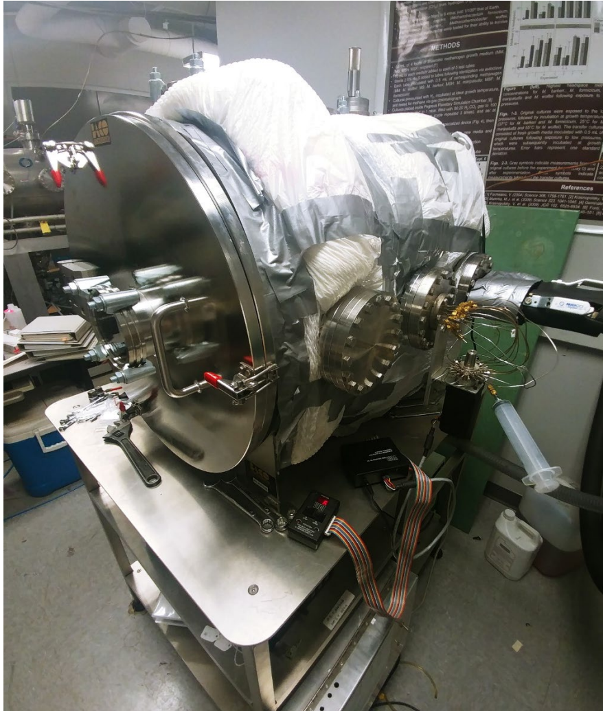
Figure 27. Pegasus biochamber at the Keck Lab of the University of Arkansas. This chamber possesses a chiller connected to a cooling plate which is positioned inside of the chamber for cold experiments. Plate is connected to a Lauda Chiller.
