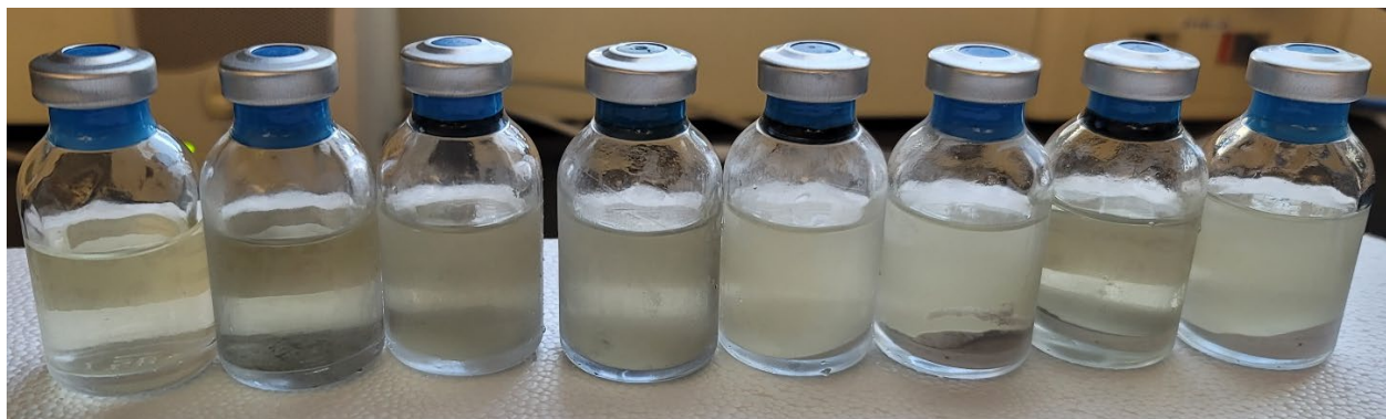
Figure 34. Cultures incubated at 10 °C for 30 days and supplemented with CaSO 4 . From left to right: Growth negative control, 0.35 wt%, 1 wt%, 5 wt%, 10 wt%, 15 wt%, 20 wt%, and 25 wt% supplementations with CaSO 4 .
