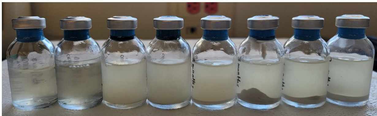
Figure 39. Cultures incubated at -10 °C for 90 days and supplemented with CaSO 4 . From left to right: Growth negative control, 0.35 wt%, 1 wt%, 5 wt%, 10 wt%, 15 wt%, 20 wt%, and 25 wt% supplementations with CaSO 4 .
