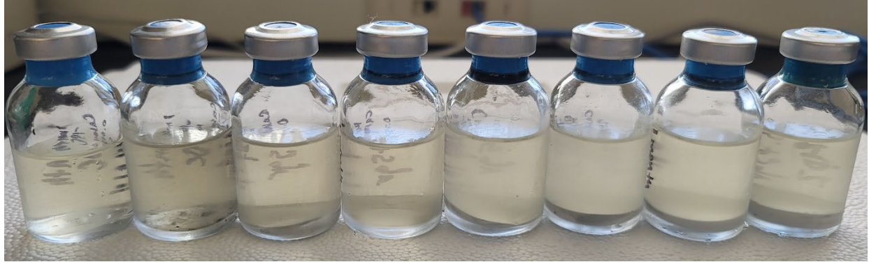
Figure 37. Cultures incubated at -5 °C for 90 days and supplemented with CaSO 4 . From left to right: Growth negative control, 0.35 wt%, 1 wt%, 5 wt%, 10 wt%, 15 wt%, 20 wt%, and 25 wt% supplementations with CaSO 4 .
