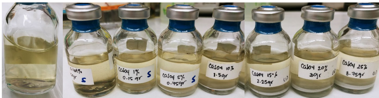
Figure 35. Cultures incubated at 10 °C for 90 days and supplemented with CaSO 4 . From left to right: Growth negative control, 0.35 wt%, 1 wt%, 5 wt%, 10 wt%, 15 wt%, 20 wt%, and 25 wt% supplementations with CaSO 4 .
