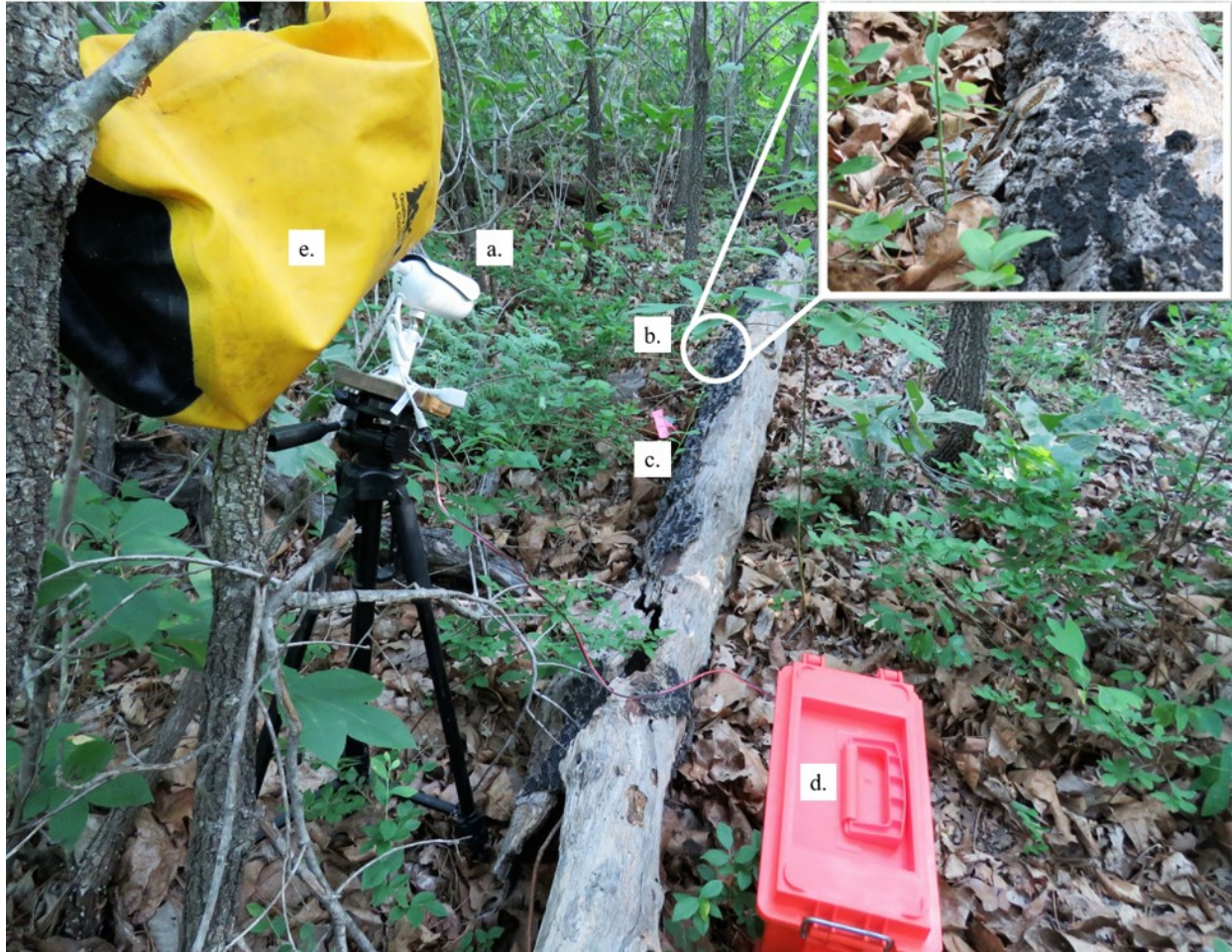
Figure 1. A typical videography setup illustrating the audio equipped surveillance video camera (a.) positioned on a snake (b.) and HOBO pendent ® data logger (c.). The battery (d.) was housed in the orange dry box and the telemetry receiver was housed in a waterproof bag (e.). The system was highly mobile, waterproof and could run continuously for approximately 36 hours depending on camera settings. However, most snakes relocated within 24 hours after camera setup, or the battery was replaced approximately every 24 hours.
