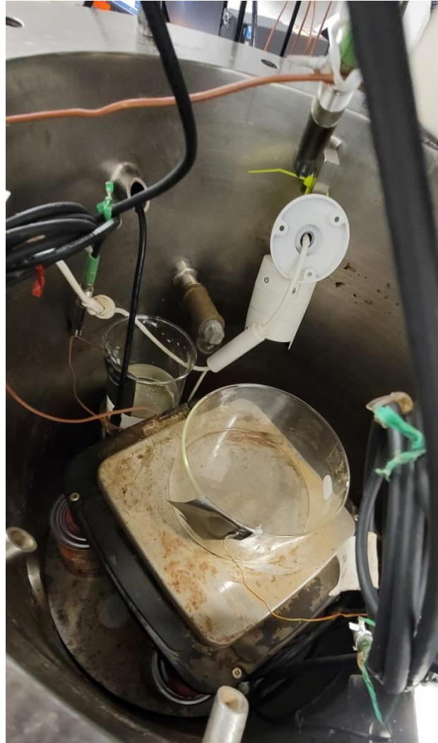
Figure 1: Inside look of the chamber with the scale and petridish elevated by four cans, one in each corner. The NaCl saturated humidity buffer is elevated on a can, so the buffer can be closer to the sample.
