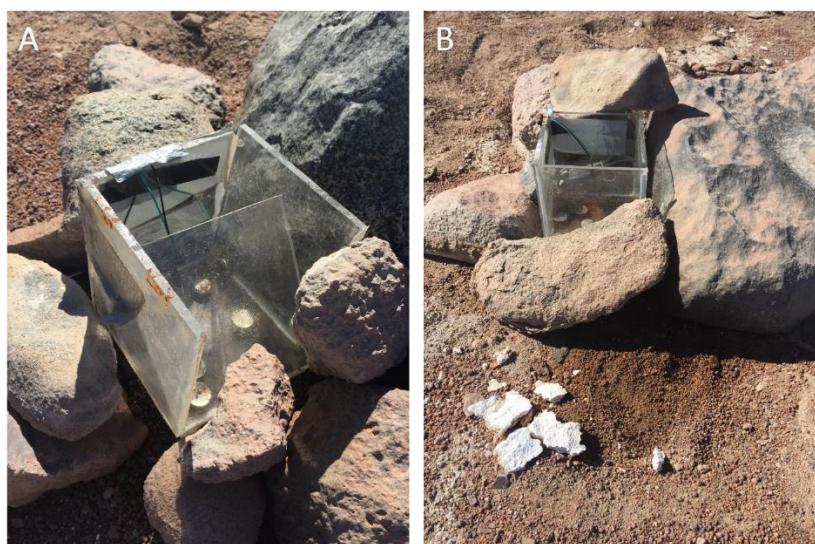
Figure 5: A: Installation of sample boxes in the field. Samples were “camouflaged” to the best of our ability by placing boxes up against small boulders and covering electronics with small rocks. B: Wide shot of the field site in Yungay showing active installation of sample box with others already set in place. (Photo credit: Holly Blann)
