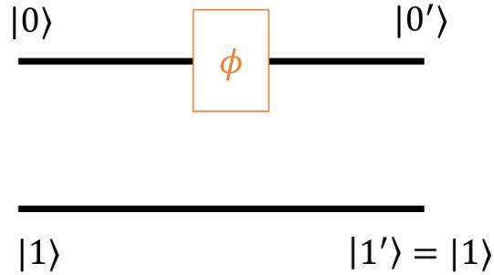
Figure 1.2 Phase Shifter Logic Gate
