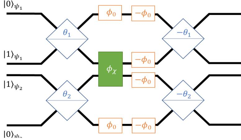
Figure 1.3 Example  $U_{CP}$  Set-up
