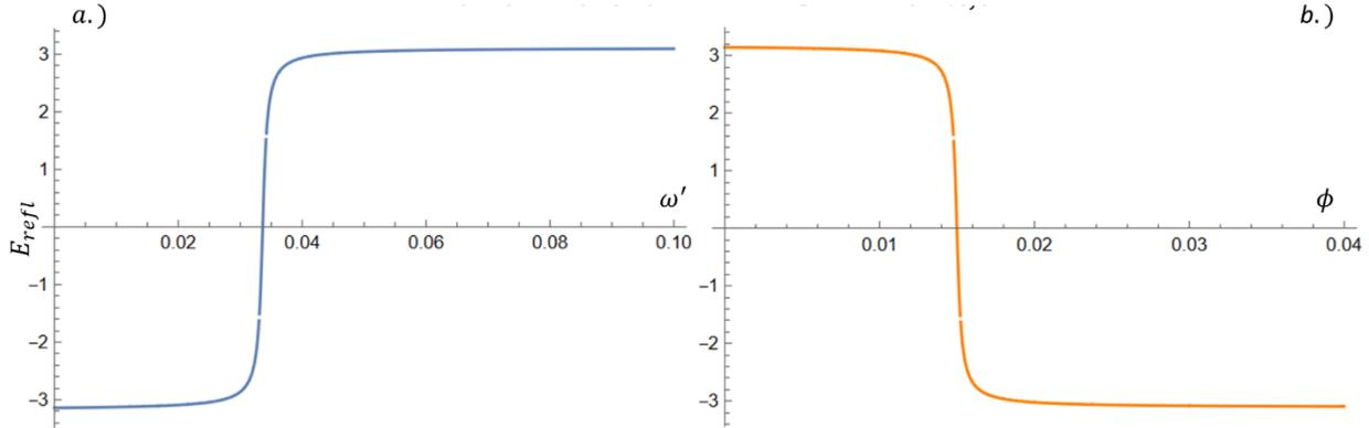
Figure 3.2 Rapid phase flip of the real argument of  $E_{refl}$
