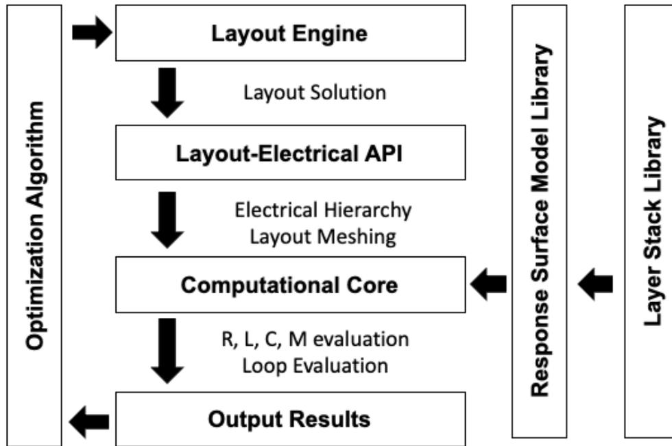
**Fig. 3.1 Layout engine to electrical evaluation API**
