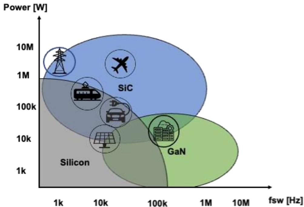
Fig. 1.1 Operating frequency versus power output for WBG devices and their application
