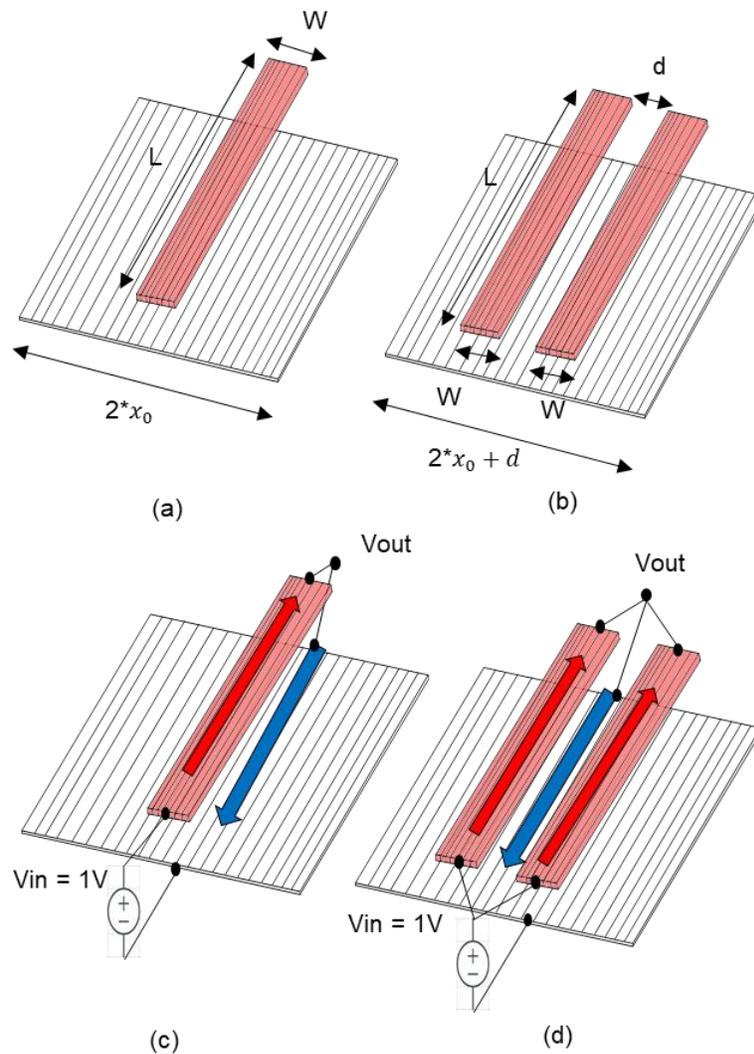
**Fig. 2.12 Input parameters for (a) a single trace (b) mutual inductance between traces, Simulation setup for (c) single trace impedance (d) mutual inductance.**
