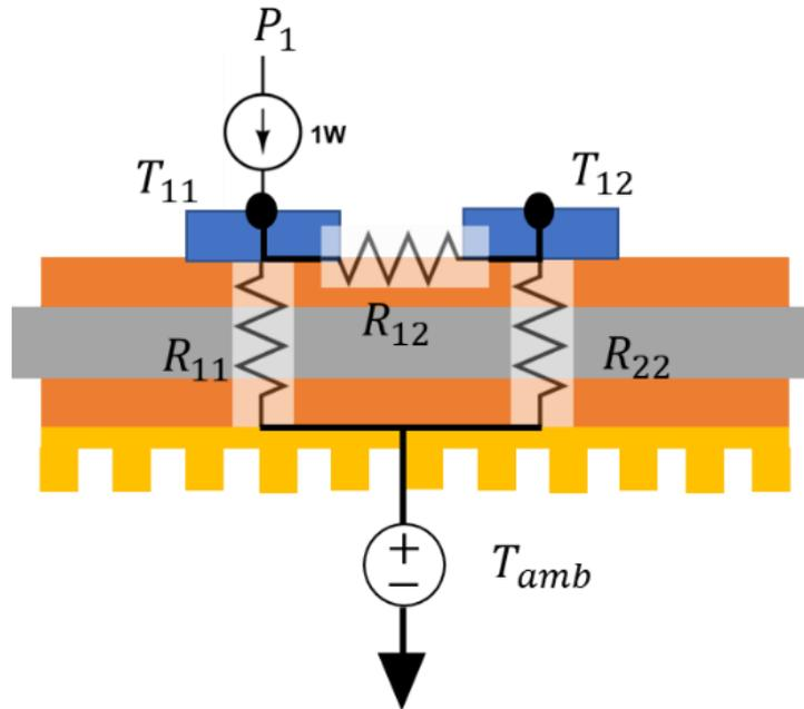
**Fig. 6.5 Example thermal network extracted from an MCPCB structure with 2 devices**
