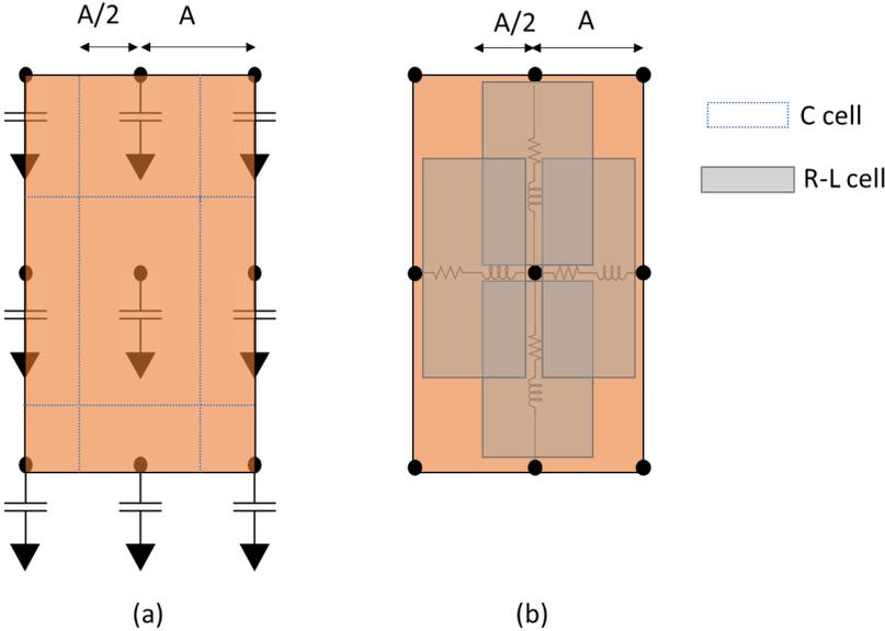
**Fig. 4.4 Different meshing cell types in PEEC (a) Capacitor (b) Resistor and Inductor**
