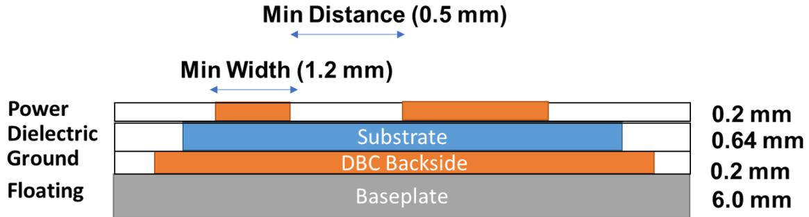
**Fig. 3.2 A layerstack representation in PowerSynth**
