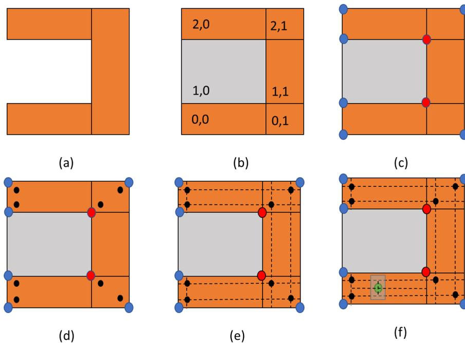
**Fig. 4.5 Meshing process of MCPM (a) input layout (b) matrix-based grid (c) detect corner types (d) adding near corner mesh points (e) trace level meshing (f) device placement**
