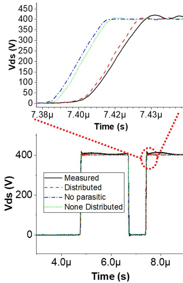
**Fig. 5.11 Waveform comparison among different simulation approaches.**
