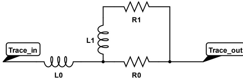
**Fig. 2.13 Ladder Circuit for Broadband Frequency Extraction**
