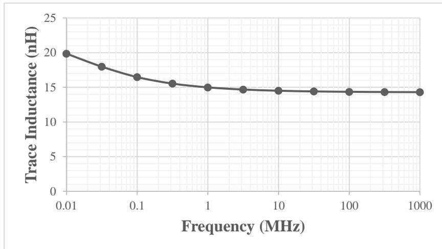
**Fig. 2.9 Inductance reduction versus frequency for an MCPM trace**
