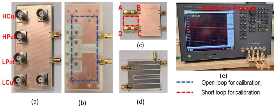
**Fig. 5.14 (a) topside of custom-made PCB fixture (b) bottom side of PCB fixture (c) board for short calibration (d) design under test layout (e) impedance analyzer.**
