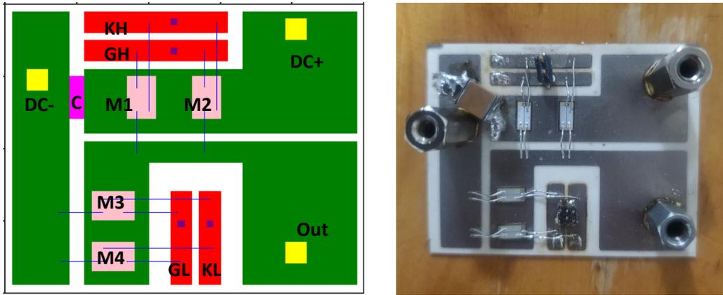
**Fig. 5.8** Generated layout from PowerSynth (left) DUT for DPT measurement (right)
