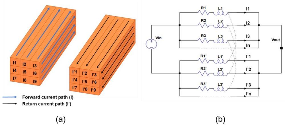
**Fig. 4.6 (a) forward and return currents for parallel traces (b) Equivalent circuit representation**
