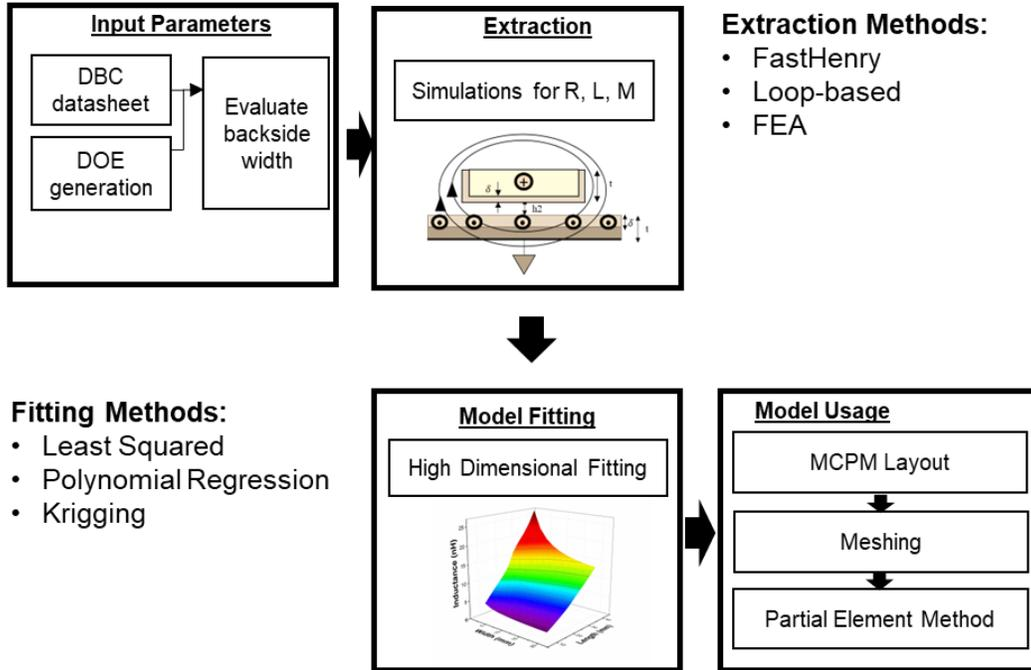
**Fig. 2.11 Extraction Process for MCPM trace model**
