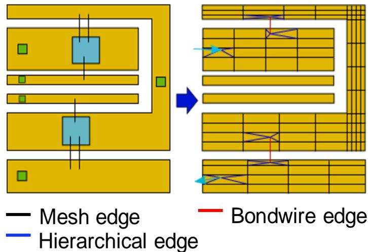
**Fig. 5.5 The uniform mesh for the structure from the previous PowerSynth hardware validation DUT**
