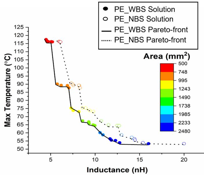
**Fig. 5.18 Pareto frontier comparison for with and without backside consideration**
