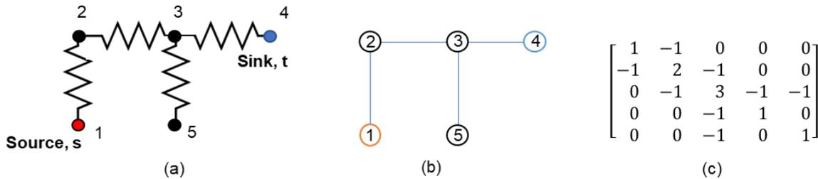
**Fig. 4.2 (a) Parasitic network, (b) Graph representation, (c) Laplacian Matrix**
