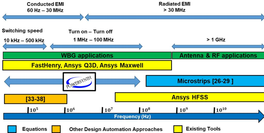
**Fig. 1.9 Different frequency range for parasitic extraction tools**
