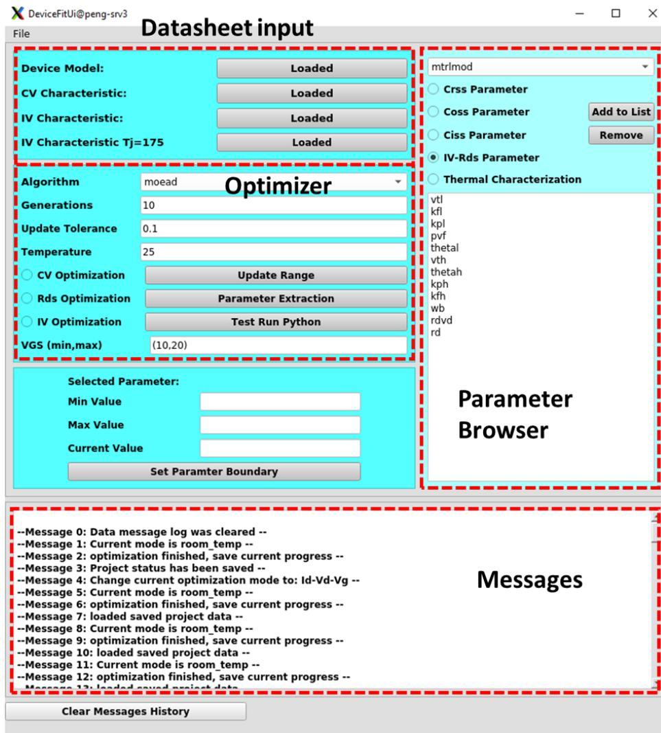
Fig. 6.3 GUI of the automate device parameters extraction tool
