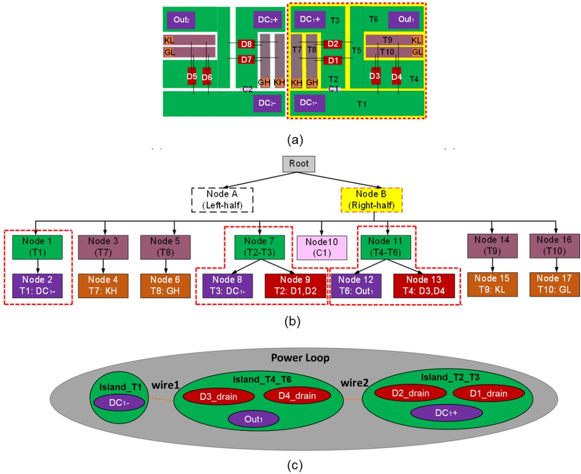
**Fig. 3.9 (a) Layout Input (b) Layout engine hierarchical tree structure (c) Power loop net in a hypergraph.**
