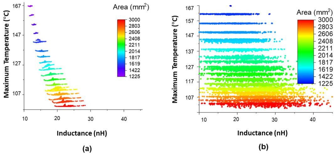
**Fig. 5.12 Solution spaces using (a) uniform meshing approach (b) optimized meshing approach**
