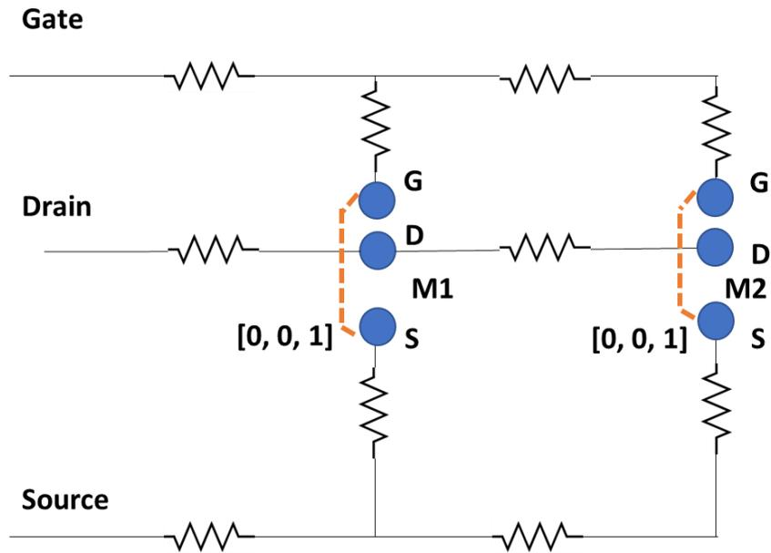
**Fig. 3.6 Gate-Kelvin loop setup for device state with gate to source connection  $[0,0,1]$**
