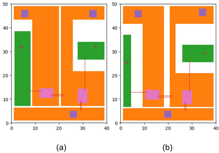
**Fig. 6.11 Two selected layouts with similar loop inductance (a) Layout 1: 10.5 nH (b) Layout 2: 10.8 nH**
