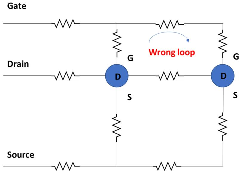
**Fig. 3.3 PowerSynth V1 device component representation**
