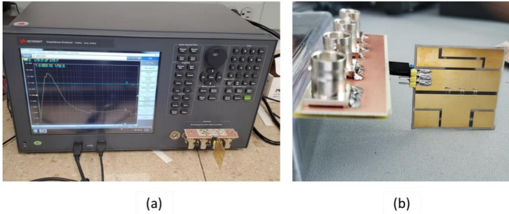
**Fig. 5.22 (a) E4990A impedance analyzer (b) Fabricated 3D DUT.**
