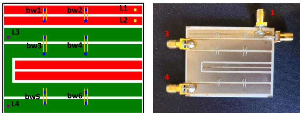
**Fig. 5.7 PowerSynth layout (left) and DUT (right) for S-Parameter measurement**
