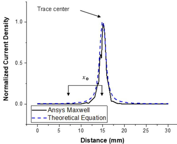
**Fig. 2.10 Normalized current density versus analytical equation**
