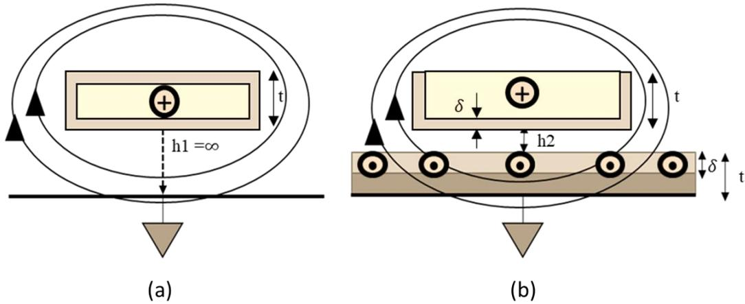
**Fig. 2.6** Cross section of the conductor trace for (a) no backside, (b) with backside, where  $h_1$  is the distance to backside,  $\delta$  is the skin-depth value, and  $t$  is the copper thickness
