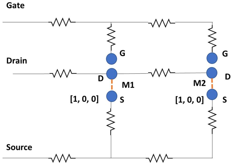
**Fig. 3.5 Power loop setup for device state with drain to source connection  $[1,0,0]$  for each device**
