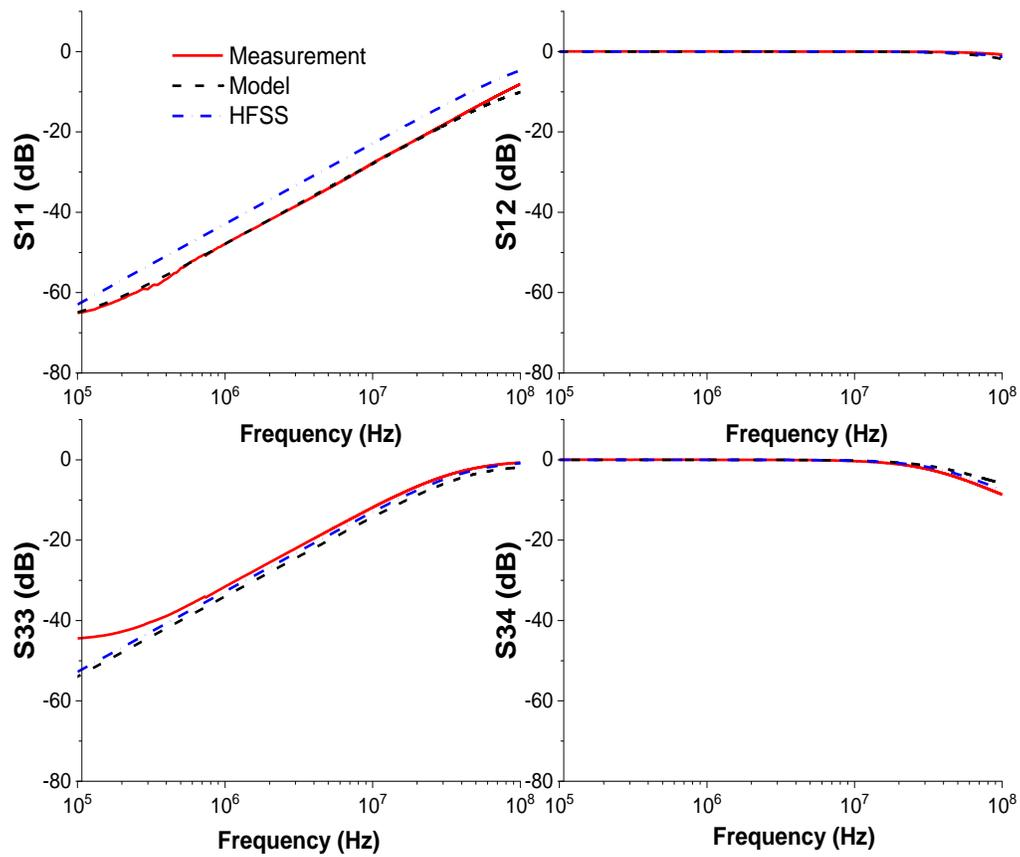
**Fig. 5.9 S-parameter measurement versus model extraction and HFSS**
