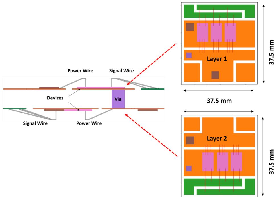
**Fig. 5.21 Side and layer-layer views of the fabricated 3D layout.**
