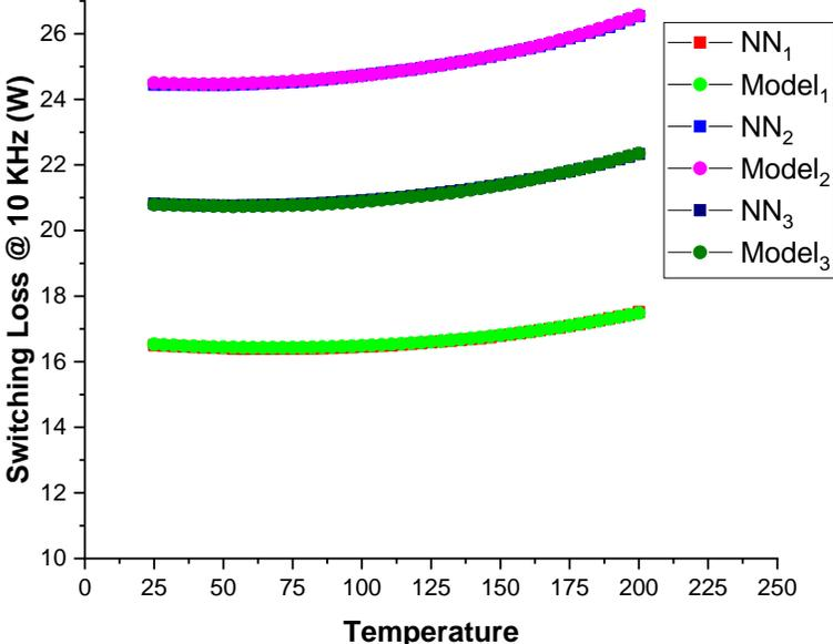
**Fig. 6.7 Fitting accuracy between the FFNN and Analytical Model**
