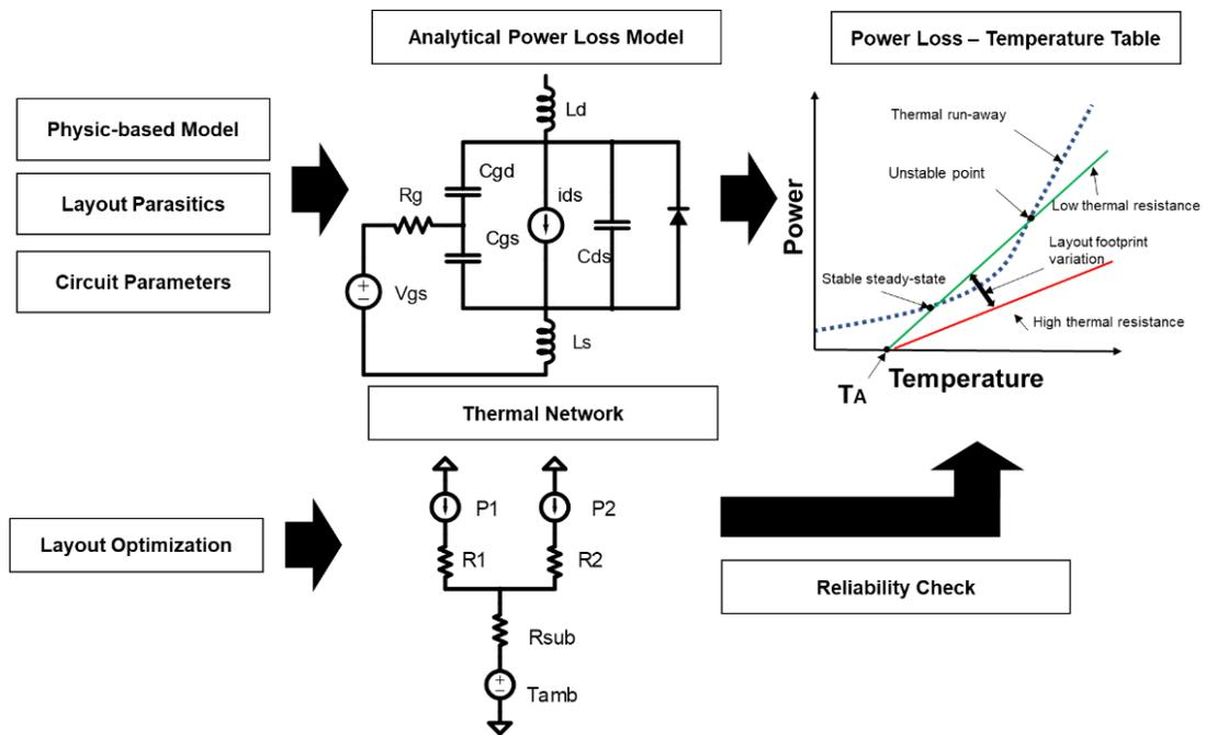
**Fig. 6.4 Electrothermal simulation for dynamic performance**
