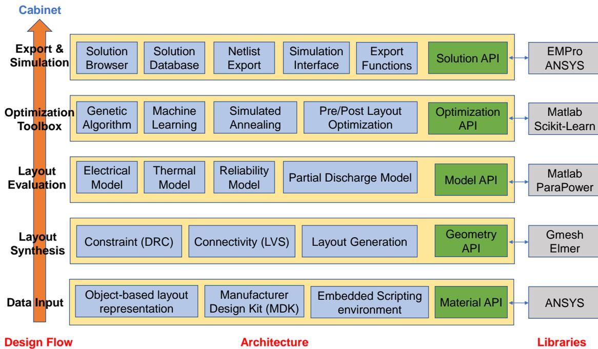
**Fig. 1.5 Software Architecture for PowerSynth v2**
