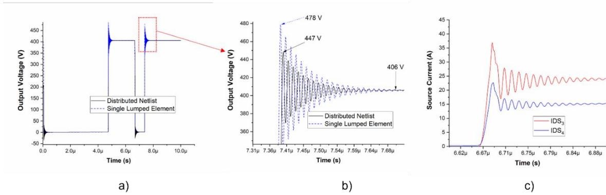
**Fig. 5.20 a) DPT VDS waveform b) Zoomed in of VDS c) Source current comparison on lower side devices.**
