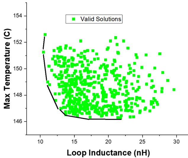
**Fig. 6.9 A common solution space obtained from PowerSynth with all valid solutions**
