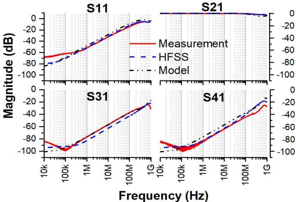
Fig. 5.4 S-parameter comparison of the 4-port DUT
