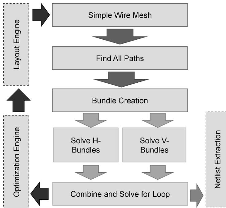
**Fig. 4.7 Layout engine to loop-based model conversion**
