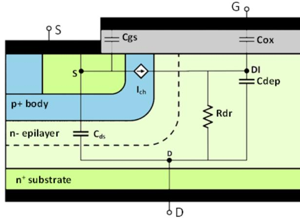
**Fig. 6.1 SiC Power MOSFET device structure with corresponding parasitic elements**
