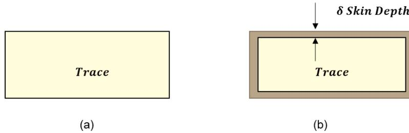
**Fig. 2.5 Cross section of a conductor trace (a) at DC range (b) at high frequency**
