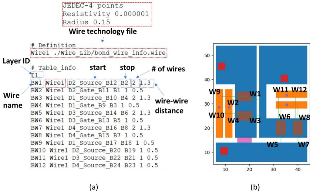
**Fig. 3.7 Bondwire (Via) connectivity input file**
