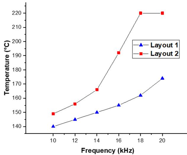
**Fig. 6.12 Comparison between 2 layout solutions with similar loop inductance values**
