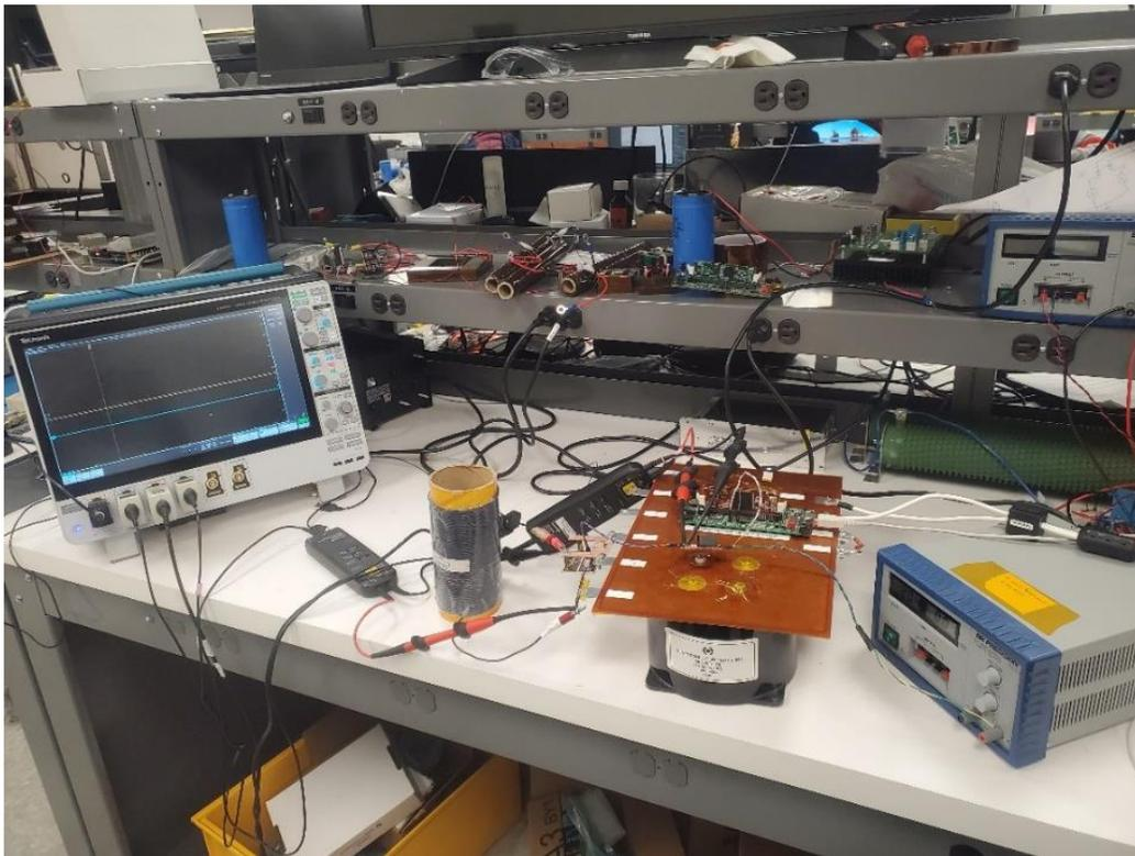
**Fig. 5.10 Experimental setup for the DPT measurement**
