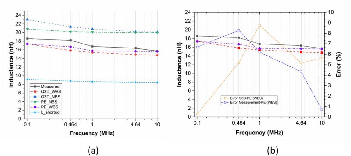
**Fig. 5.15 (a) Comparison among different methods and measurement (b) Error comparison among measurement and models with backside consideration.**
