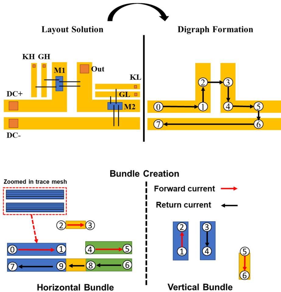
**Fig. 4.8 Layout to bundles transformation process**
