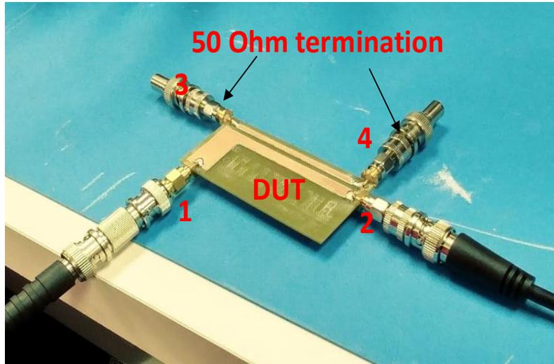
Fig. 5.3 PCB structure for 4 -port measurement
