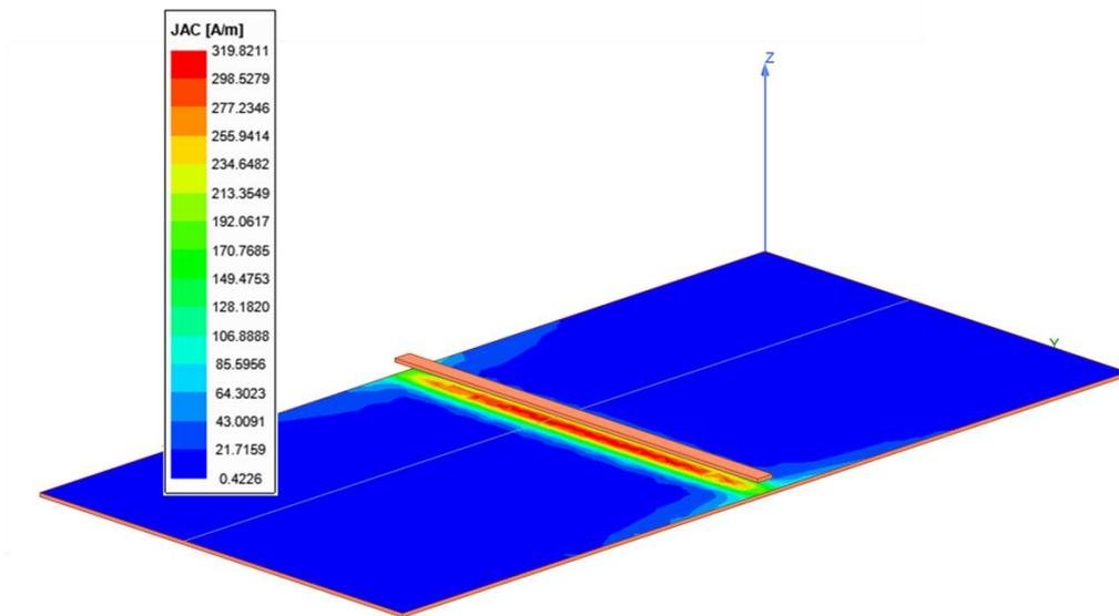
**Fig. 2.7 MCPCB trace with current density plotted on the backside copper**
