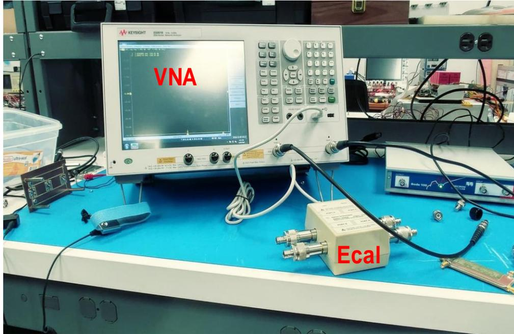
**Fig. 5.2 Vector Network Analyzer for S-Parameter measuring**
