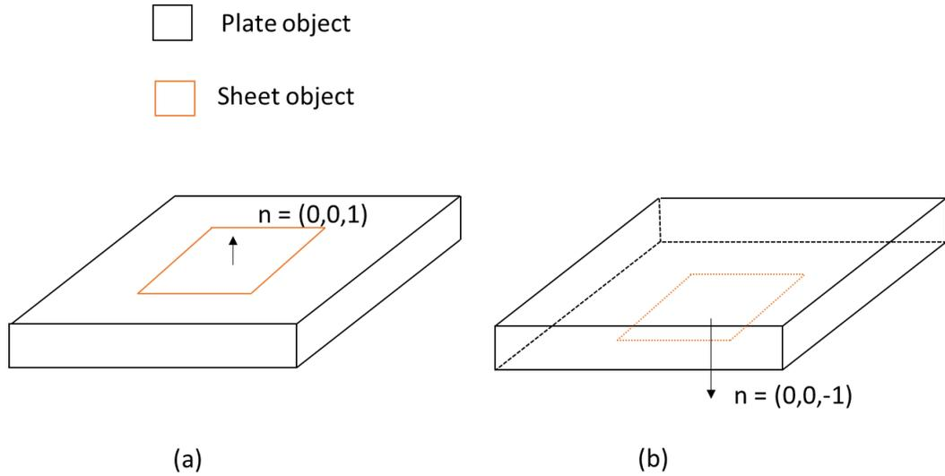
**Fig. 3.8 face-up (a) and face-down (b) positions for a sheet object**
