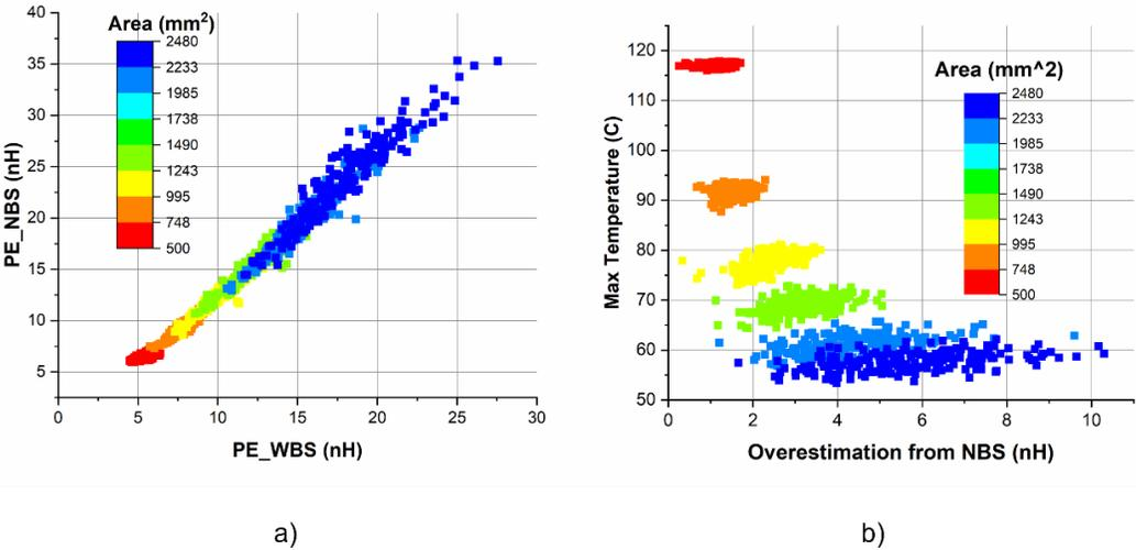
**Fig. 5.17 (a) Direct comparison between 2 approaches (b) Absolute difference between 2 approaches versus maximum temperature.**
