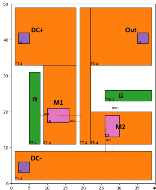
**Fig. 6.8 Half-bridge MCPM layout for the study**
