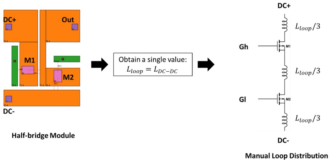
**Fig. 4.9 The manual netlist extraction method**
