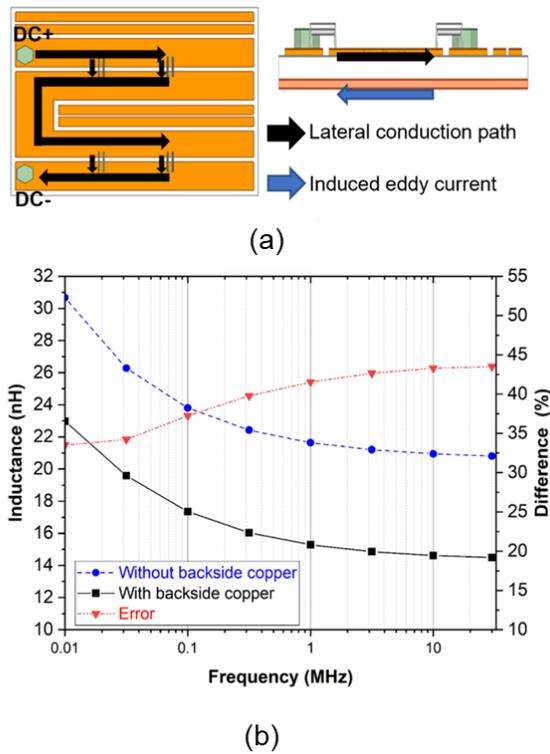
**Fig. 1.8 (a) lateral versus eddy current paths (b) eddy current impact on MCPM layout**
