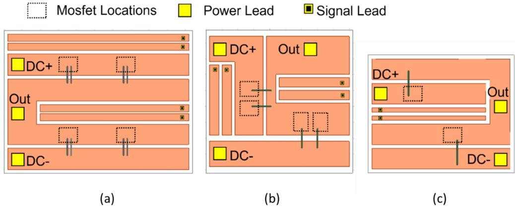
**Fig. 5.16 Selected Layout for Comparison versus FEA**
