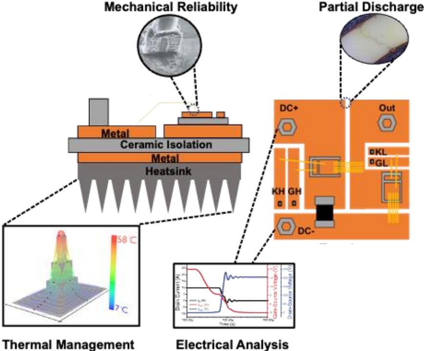
**Fig. 1.2 Design consideration for a conventional MCPM layout**
