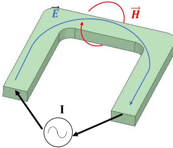
**Fig. 2.1 A time varying current in a loop.**
