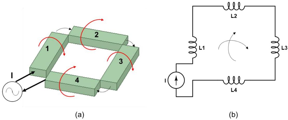
**Fig. 2.3 (a) Multiple connected loops (b) Circuit representation**
