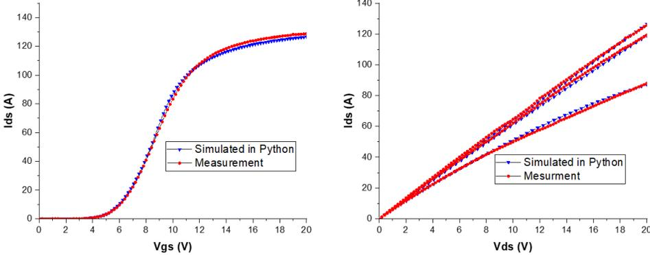
**Fig. 6.2 Measurement vs fitting results of SiC MOSFET at room temperature**
