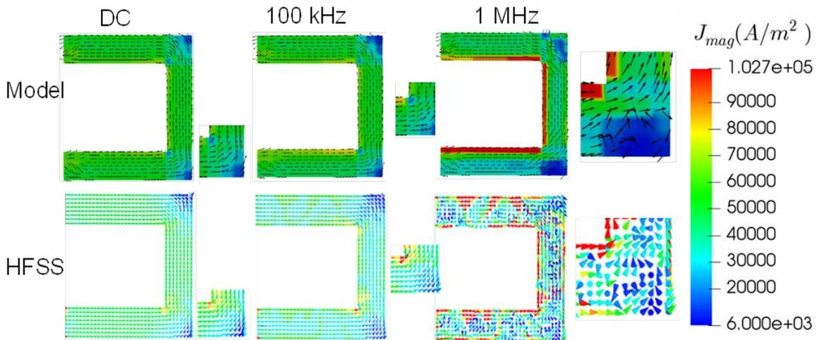
**Fig. 5.1 Current Density verification for increasing frequency**
