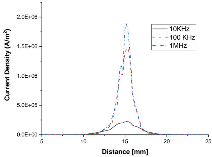
**Fig. 2.8 Eddy current density with increasing frequencies**
