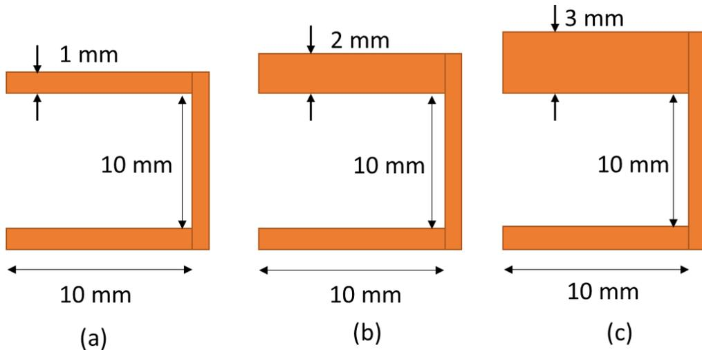
**Fig. 4.3 Different U-shape configurations**
