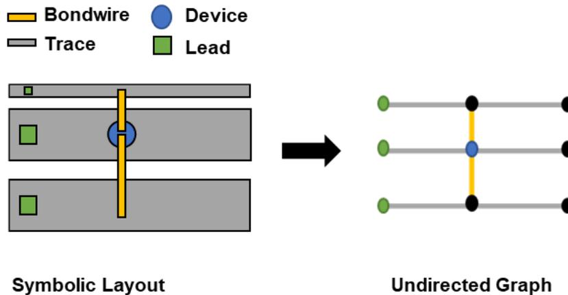
**Fig. 4.1 Symbolic layout and undirected graph representation**
