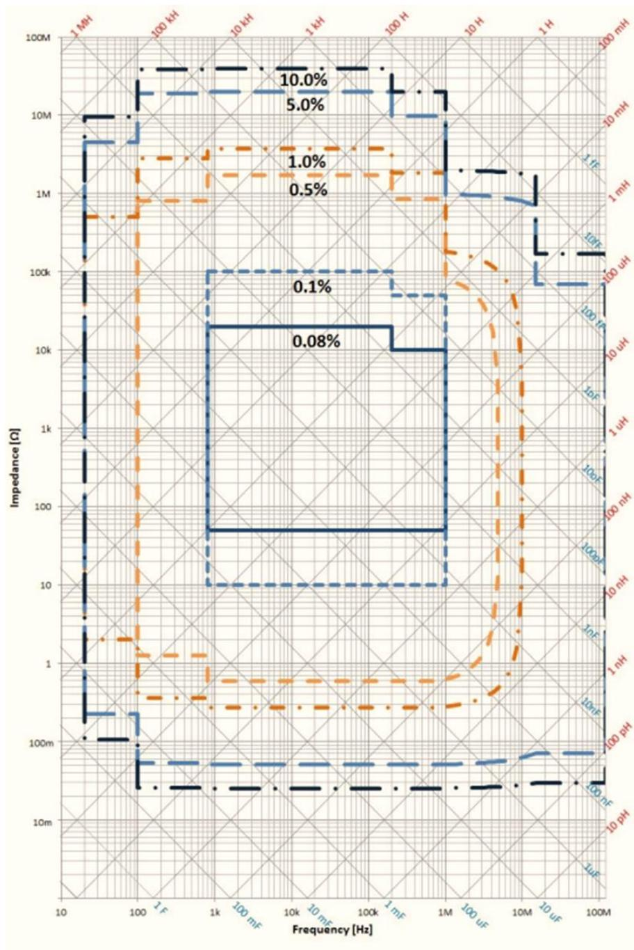
**Fig. 5.13 Accuracy range versus frequency and impedance value for E4990A**
