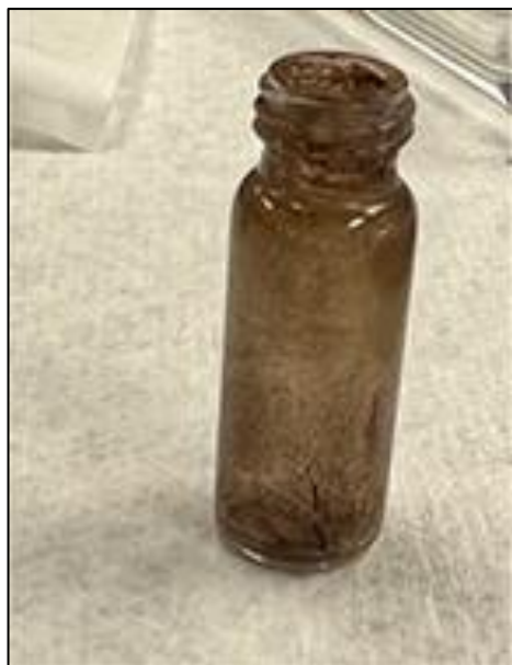
Figure 4: Tholins and hexane sample after the transfer of the liquid into the cuvette. The soild brown residue left behind show the adhesion of the tholin to the glassware.
