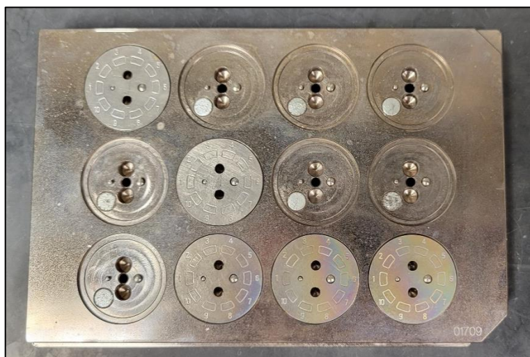
Figure 9: MALDI sample disks placed into holding tray after tholin deposition. Tholins were produced for 1 hour (middle left disk), 4 hours (lower left disk), 6 hours (lower middle disk), and 12 hours (lower right disk). The control disk is located on upper right corner.
