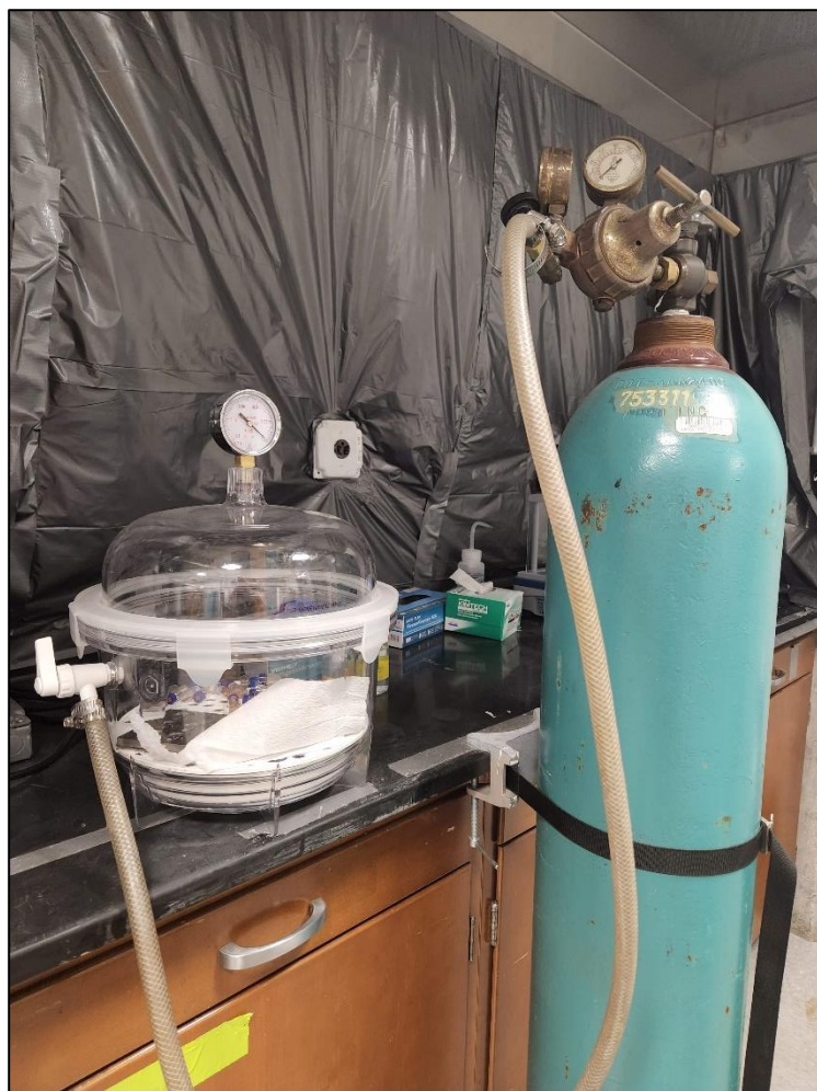
Figure 8: Tholin storage apparatus utilized. A sealed desiccator is kept at room temperature under argon (Ar) limiting the organics' potential reaction with ambient oxygen (O 2 ) and water (H 2 O).
