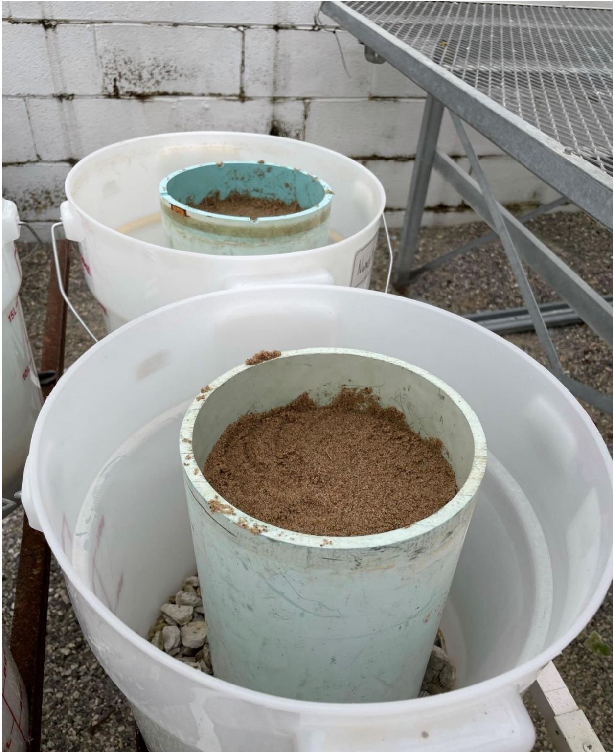
Figure 4.1. An example of a PVC lysimeter packed with 20 cm of sand placed on 10 cm of gravel within a beverage dispensing bucket to investigate the effect of subsurface nanobubble-oxygenated irrigation water on creeping bentgrass growth.
