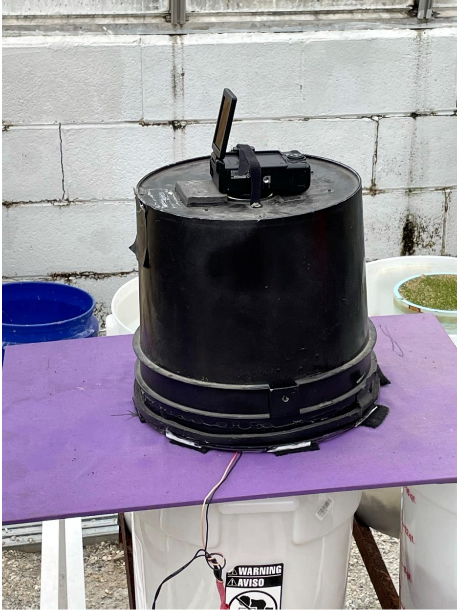
Figure 4.4. Modified light box used to capture images digitally analyzed for green turfgrass coverage and the dark green color index of creeping bentgrass grown in sand-based lysimeters.
