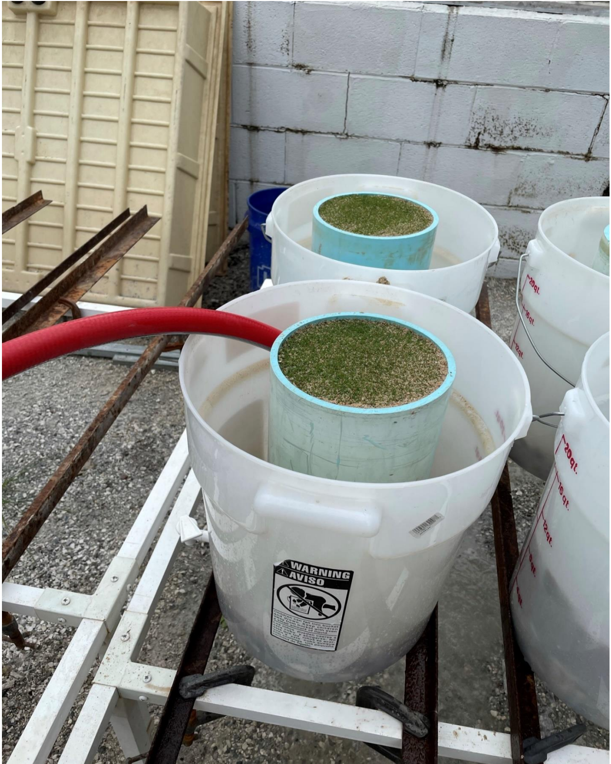
Figure 4.3. Nanobubble-oxygenated irrigation water being applied directly from the nanobubble generator to the subsurface irrigation beverage dispenser (through the red hose, center left) to investigate the effects of nanobubble-oxygenated irrigation water on creeping bentgrass grown in sand-based lysimeters.
