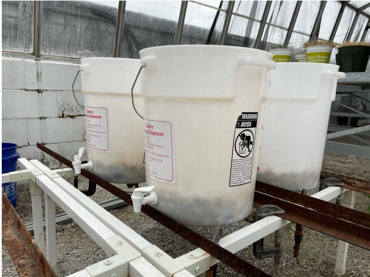
Figure 4.2. Beverage dispensers with spigots filled with 10 cm of gravel used for subsurface irrigation of creeping bentgrass grown in sand-based lysimeters with nanobubble-oxygenated irrigation water.
