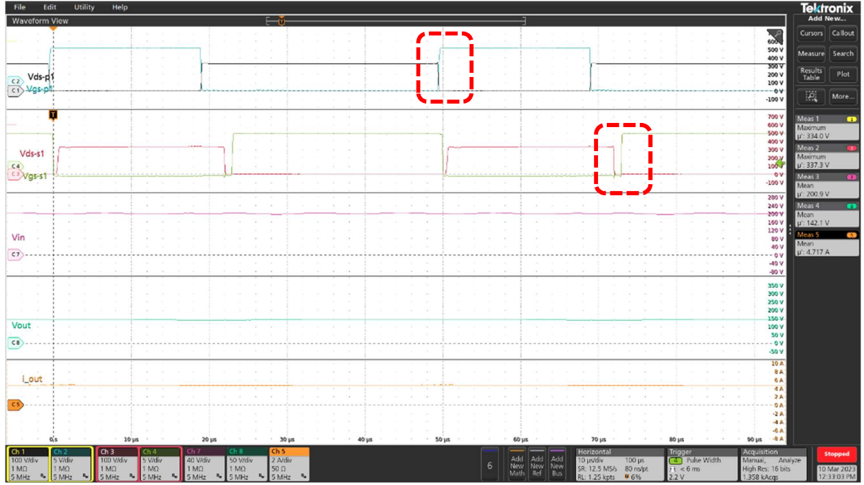
Fig. 4.6: ZVS turn-ON of the main devices S_{P1} (top), S_{S1} (second), input voltage (third), output voltage (fourth), and output current (bottom) at V_{in} = 200 V.
