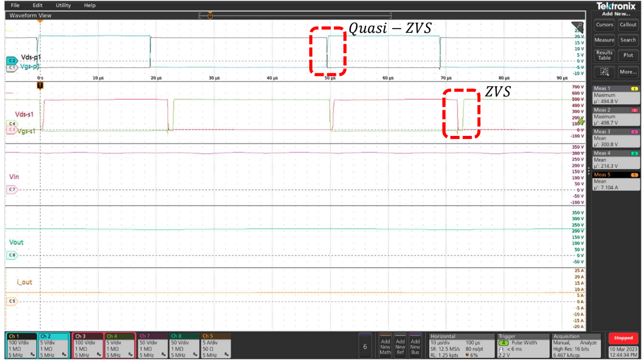
Fig. 4.7: ZVS turn-ON of the main devices S_{P1} (top), S_{S1} (second), input voltage (third), output voltage (fourth), and output current (bottom) at V_{in} = 300 V and G = 0.71 .
