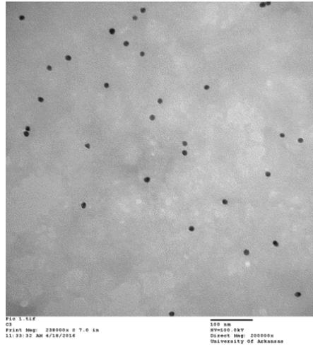
**Figure 3** TEM image of citrate Au nanoparticles.
