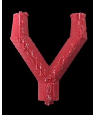
Figure 7. This figure is a photo of prototype seven. The dimensional limit of the MakerBot was not small enough causing inaccurate printing.
