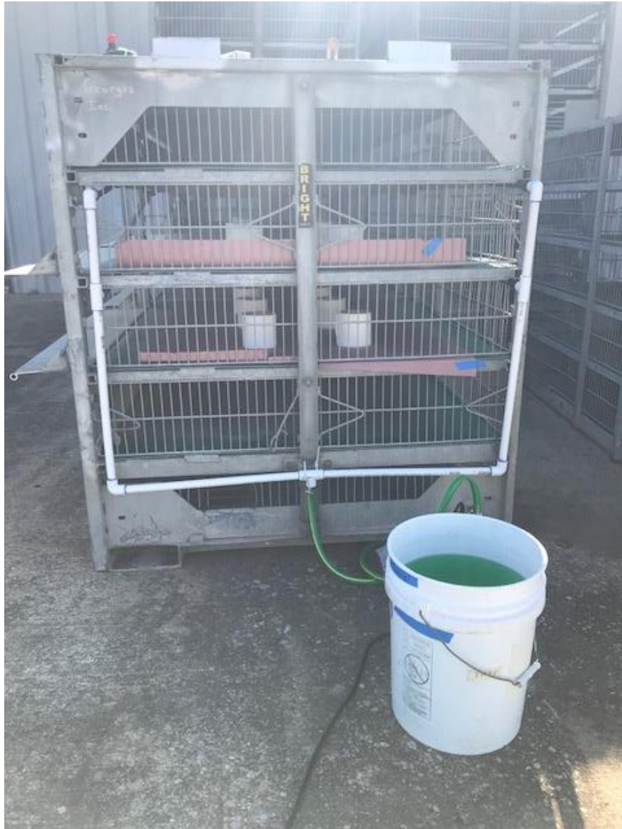
Figure 4: Prototype PVC skeleton attached to the side of the cage, with irrigation tubing extending into levels 3 and 4.
