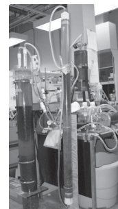
Figure 1. Photograph of Multimedia Filter
