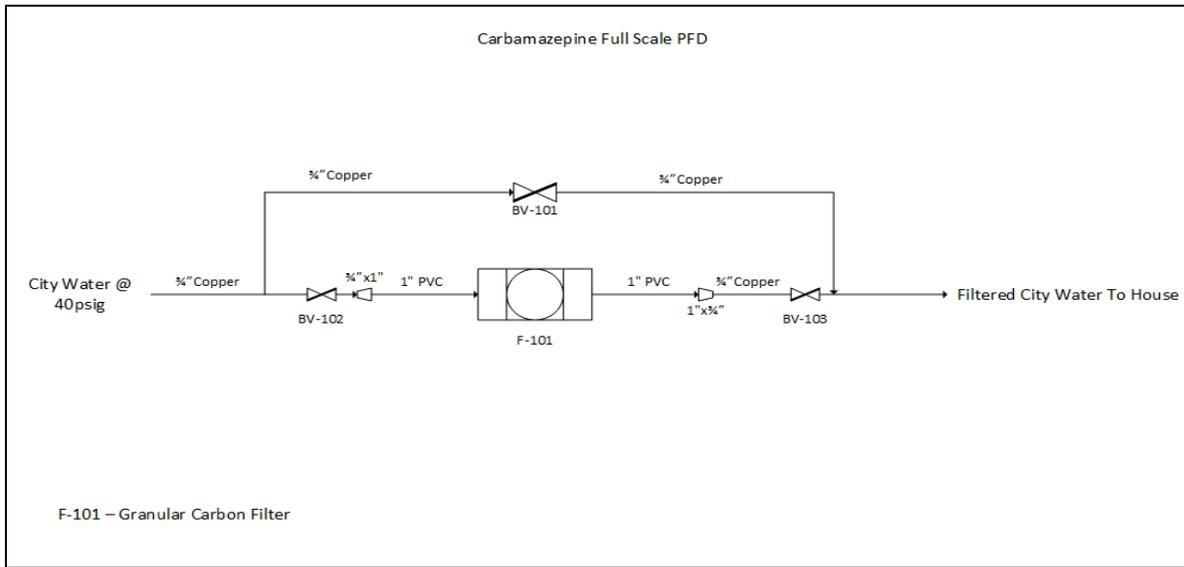
Figure 9.2.1 Home Unit Process Flow Diagram
