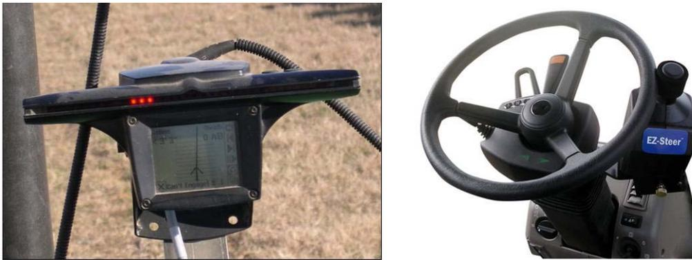
Fig. 1. Light-bar (left) and assisted-steering (right) guidance systems.
