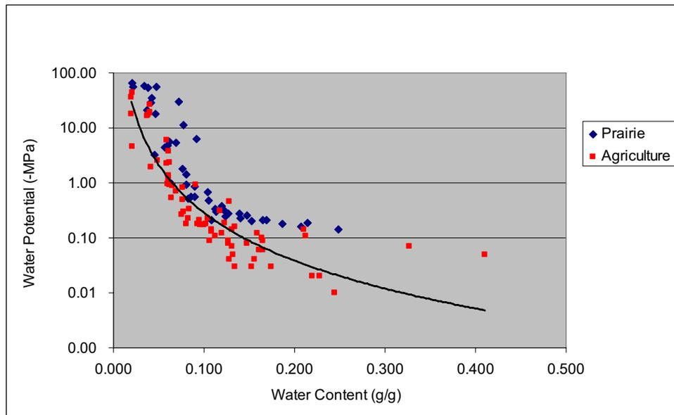
**Fig. 1.** Relationship between water potential, plotted on a log scale, and gravimetric water content for a prairie versus an agricultural soil in eastern Arkansas. The single line indicates no land-use effect on water-retention characteristics.
