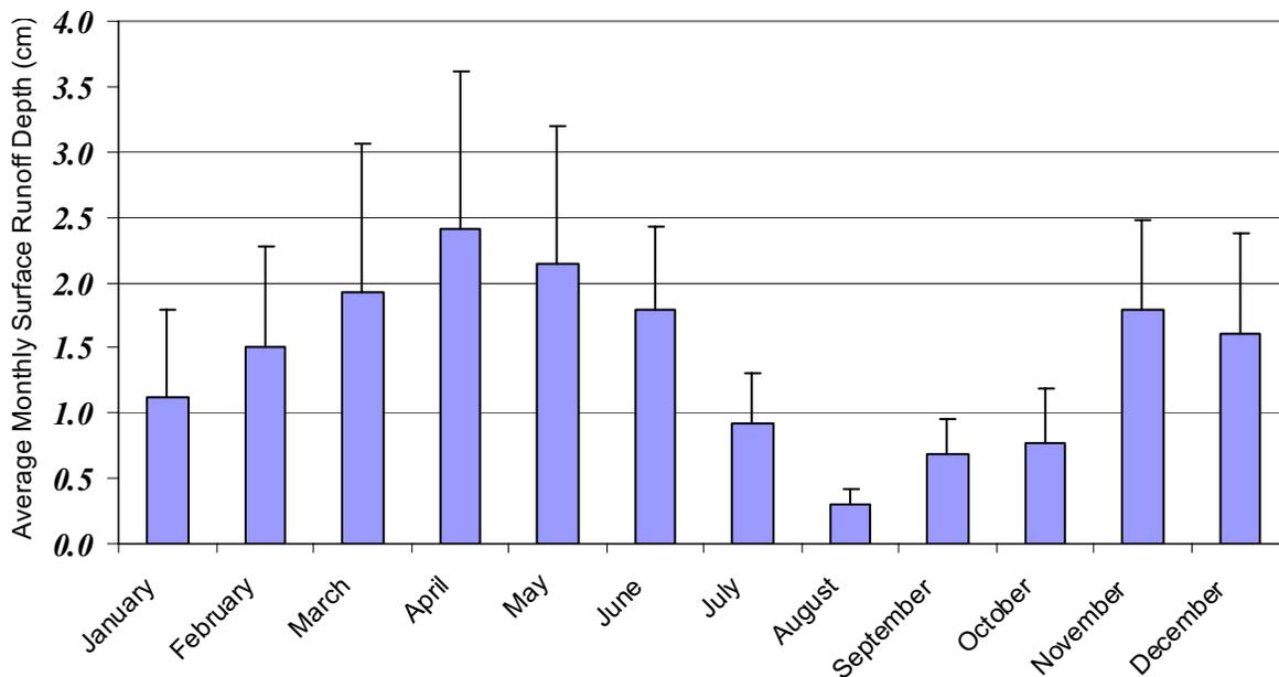
**Fig. 1.** Average monthly surface-runoff depth (cm) and standard error as calculated using daily streamflow data and hydrograph separation using the Base Flow Index software program for nine sub-basins within the Illinois River Basin, Arkansas and Oklahoma.
