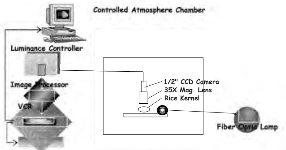
Fig. 1. Schematic of the video microscopy system.
