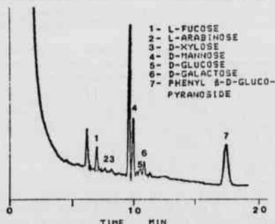
Figure. Gas chromatographic separation of neutral sugars from *C. atrox* venom as aldononitrile acetates. The initial hold was at 170° for two minutes followed by an increase of 8°/min to a final temperature of 240°. Nitrogen flow rate was 24 ml/min and sample size was 4 μl.
