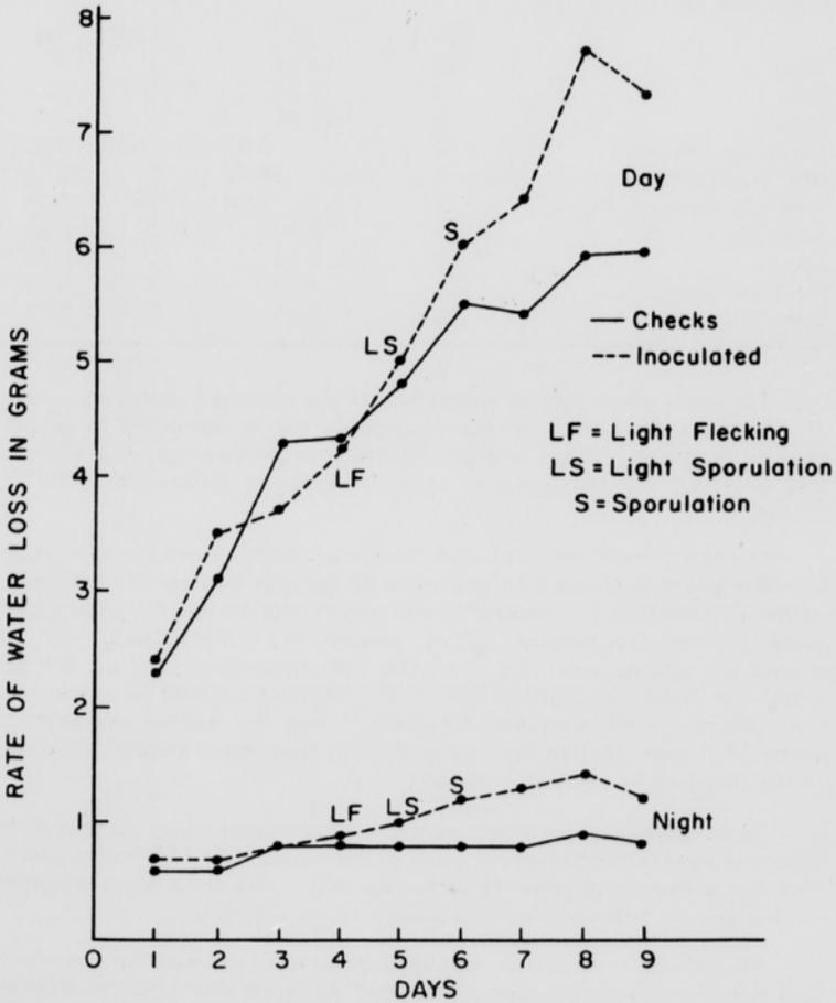
Figure 1. The effect of crown rust 216 and time on the day and night water loss of plants of the susceptible variety LEE. Graph constructed from averages of four experiments.
